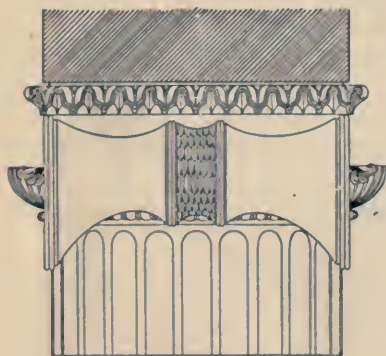
FIG. 29.—SIDE VIEW OF IONIC CAPITAL.
