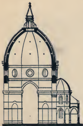
FIG. 159.—SECTION OF DOME OF DUOMO, FLORENCE.
