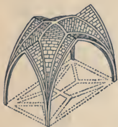
FIG. 108. — RIBBED VAULT, ENGLISH TYPE, WITH DI- VIDED GROIN-RIBS AND RIDGE-RIBS.
