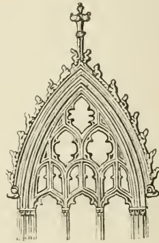
FIG. ff .—LATE PERPENDICULAR WINDOWHEAD.
