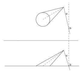
Draw a tangent line from the base of the cone in top view that goes through point b. Bring down the point where the tangent line hits the circle to the front view.
