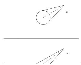
In front view, draw a line connecting the top of the cone to point a. Bring down the line to the ground. Bring up the intersection point between the line and the ground line up to top view.
