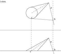
Draw a line from point C to the the top of the cone
