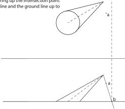
In top view, draw a line that passes through point a and that intersects the vertical line from point b.
