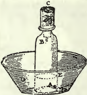
Fig. 3. Scheele's apparatus showing bees in the upper chamber of a glass apparatus filled with oxygen.
