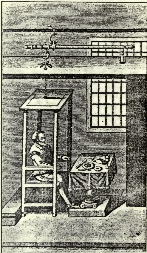
Fig. 1. Frontispiece of "De medicina statica aphorismi," showing Sanctorius seated on a chair suspended from a large steelyard.
