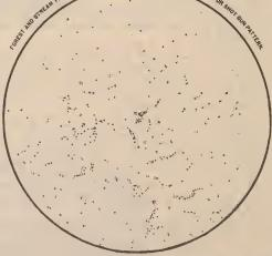
REM. 16-GAUGE, DEAD SHOT POWDER, LEFT BARREL, 232 PELLETS
