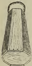
Box for one set (or nest) of pails, with rope handle. Sides \frac{1}{2} in. thick, bottom and top \frac{3}{8} inch thick.
