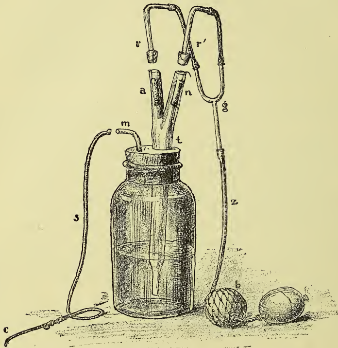
FIG. 80.—APPARATUS FOR CHLORIDE OF AMMONIUM VAPOUR.
