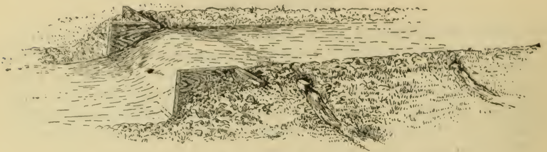
FIG. 12.—Check in head ditch and distribution of water through wooden tubes.
