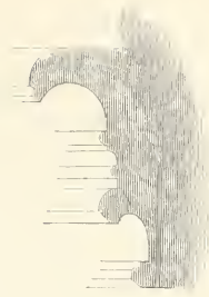
Mouldings of Capital of Chancel-Arch.
