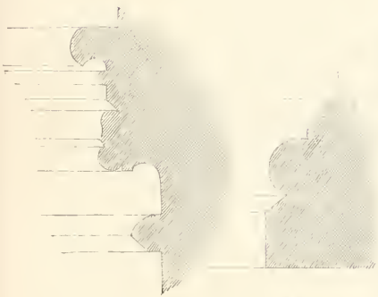
Capital and Base of a Pillar in the Nave.
