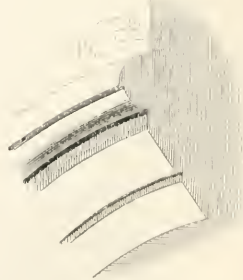
Label and Jamb of the East Window of South Chapel c. 1330
