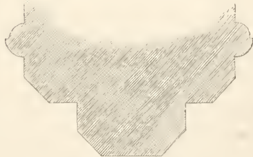
Mouldings of Chancel arch
