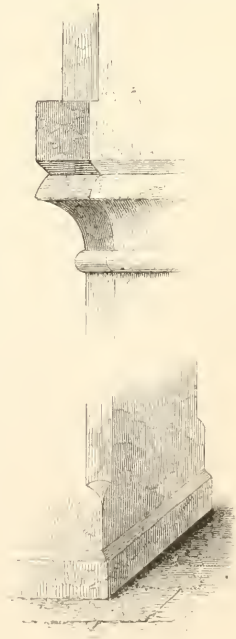
Cap and Base of Pillar in Nave.
