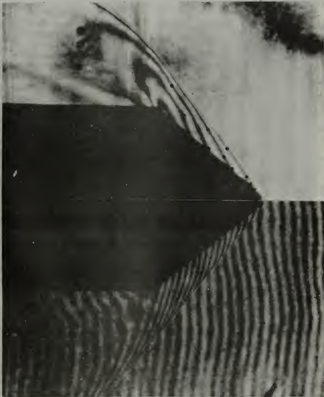
INTERFEROGRAM OF 40° CONE AT MACH 2.7; INFINITE AND FINITE FRINGE. DOTS REPRESENT VARIABLE DENSITY SOLUTION OF FRINGE PREDICTION.
