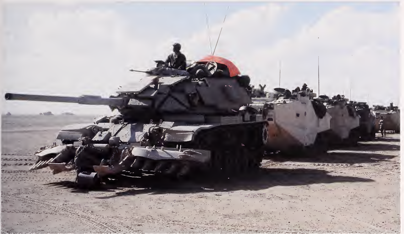
M-60A1 main battle tank equipped with reactive armor, mine-clearing rollers and plow stand by at the head of a column of AAVP-7A1 assault amphibian vehicles as I MEF prepares to enter Kuwait at the start of the ground phase of Operation "Desert Storm".
