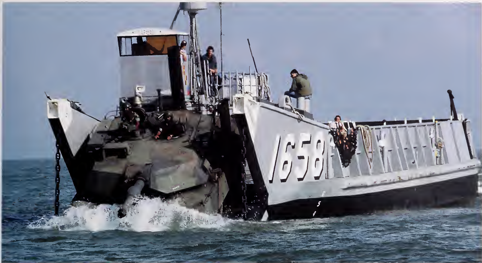
M-1A1 Abrams main battle tank enters the water from the open ramp of a utility landing craft LCU-1658. Tank is equipped with a fording kit that is being evaluated by the Marine Corps at the Naval Amphibious Base, Little Creek, VA.
