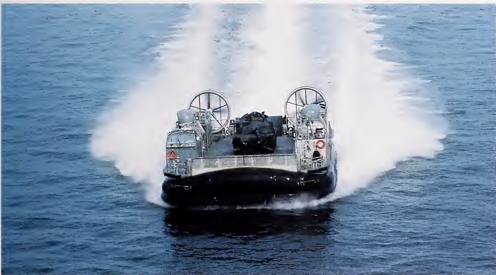
A bow view of an air cushion landing craft LCAC-12 underway near the Naval Amphibious Base, Little Creek, VA. The landing craft is carrying an M-1A1 Abrams main battle tank.
