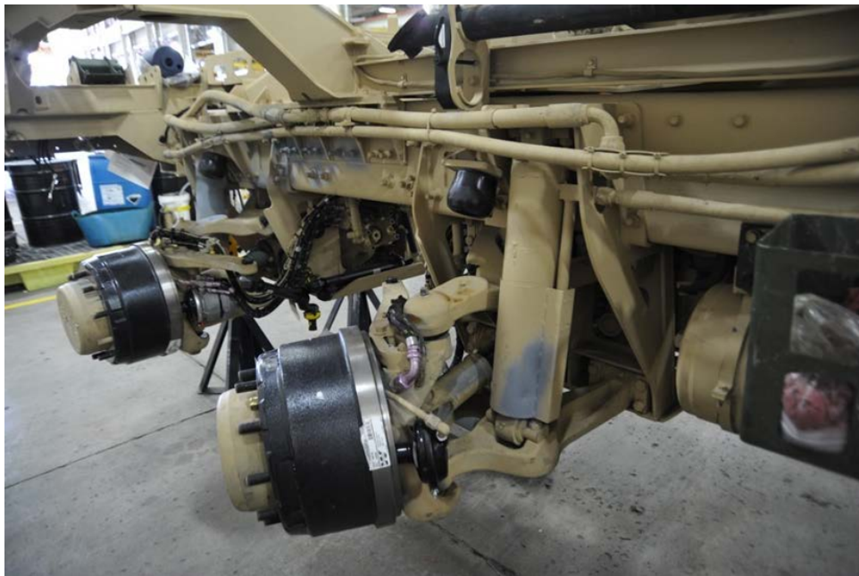
Figure 11. View of Cougar axles mounted to V-shaped hull
