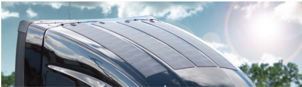
Figure 16. Flexible solar array applied to roof of commercial truck
