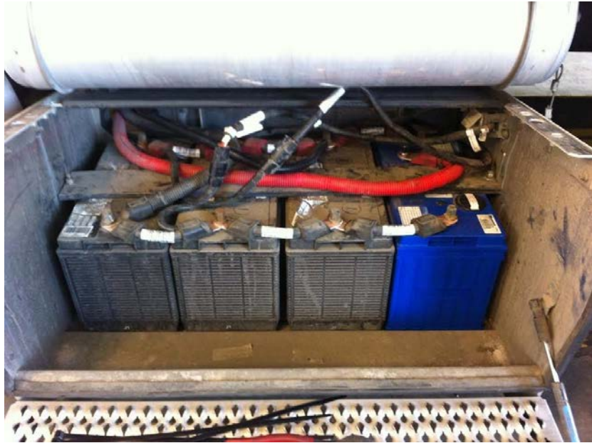
Figure 13. Visual of drop-in capacitor battery from Maxwell. Source: Amazon.com (2018).
