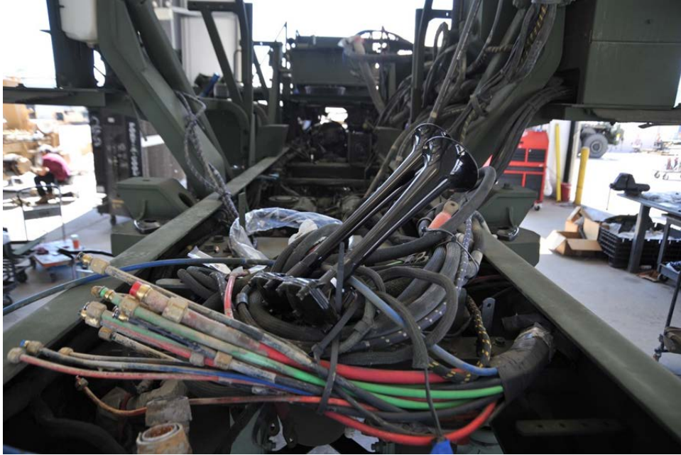
Figure 4. View of back of LVSR stripped at MCLB Barstow with cables ready for installation
