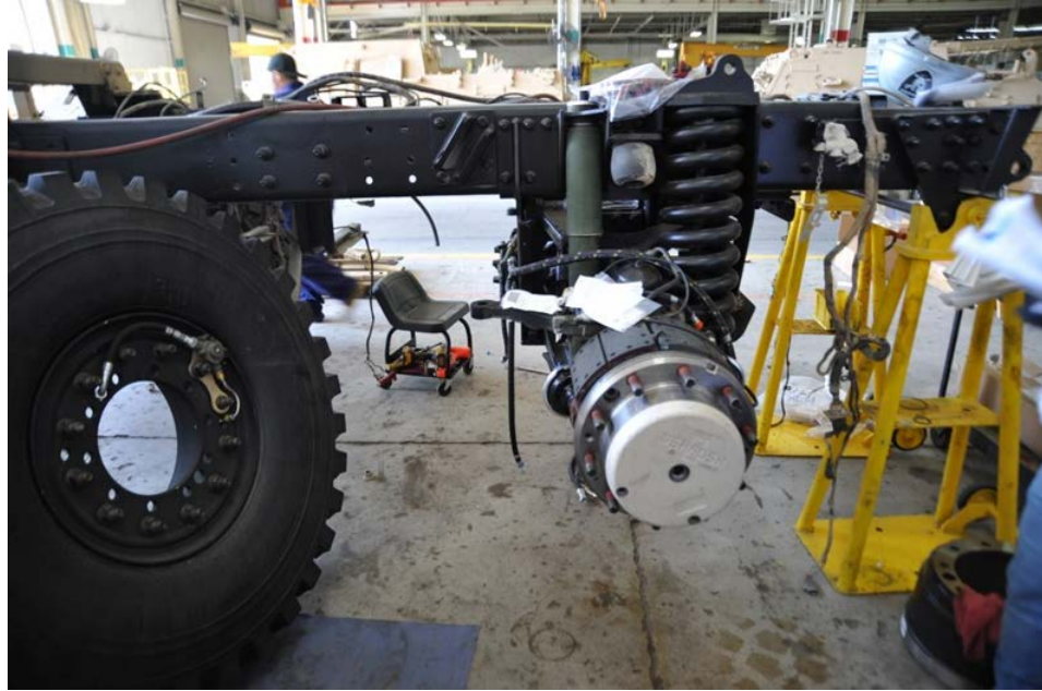
Figure 10. Side view of MTVR rear wheel axle and strut
