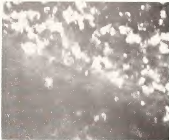
Figure 7. Dark field image of one of the Cu 2 O spots in the transmission electron diffraction pattern showing the distribution of the oxide. The area is the same as figure 6.
