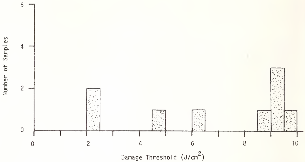
Figure 3. Laser-damage thresholds (0.6-ns, 355-nm) of porous silica antireflection coatings 80-90 nm in optical thickness. The coatings were fabricated at Livermore.
