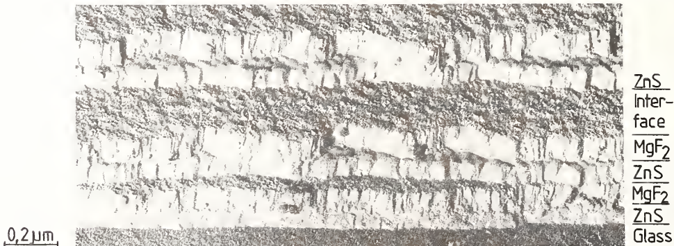
Figure 10. TEM-micrograph of the Pt/C-replica of a ZnS/MgF 2 multilayer cross-section, showing nearly amorphous microstructure for the ZnS layer next to the substrate, whereas the further ZnS layers exhibit a columnar microstructure.
