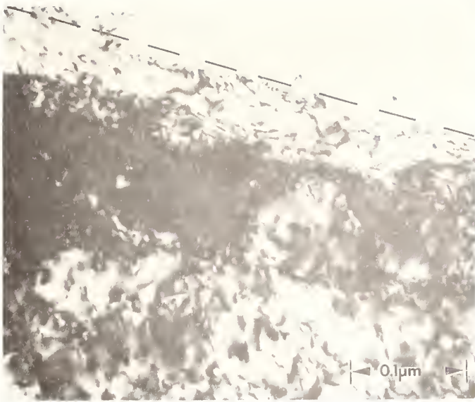
Figure 2. Bright field micrograph of the transverse section of the -5 deg rake surface. The dashed line is the boundary between the sample (lower) and the Cu electroplate (above).
