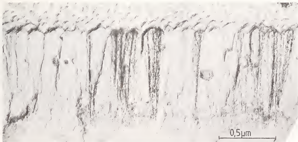
Figure 3. Fibrous substructures in TiO_2 thin films, disclosed by incomplete dissolution of actual film substance remaining on the carbon replica.
