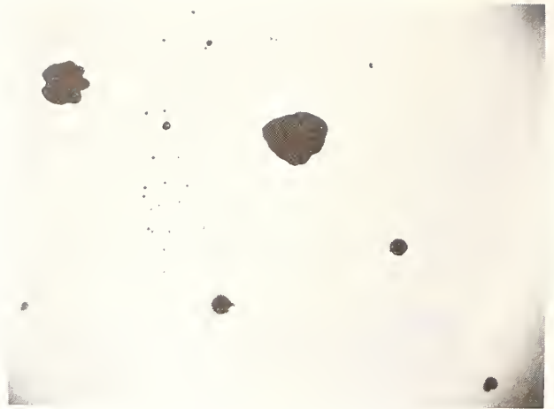
Figure 12 : Damage to a dielectric coating, 1.064 \mu\text{m} X1000 Figure 13 : Damage to PMMA, 1.064 \mu\text{m} X30
