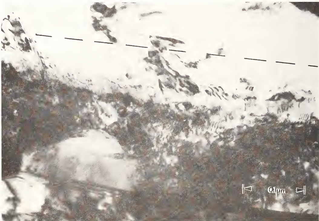
Figure 10. Transverse view of the -15 deg sample. The dashed line marks the boundary between the plating (above) and the sample.
