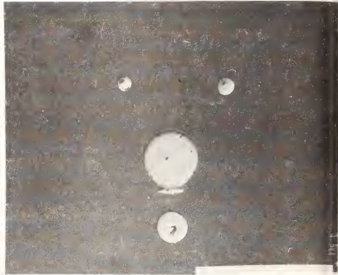
b. Single 22.5 \text{ J/cm}^2 pulse on the half wave tantalum oxide coating with electrodes. Bar is 100 \mu\text{m} .
