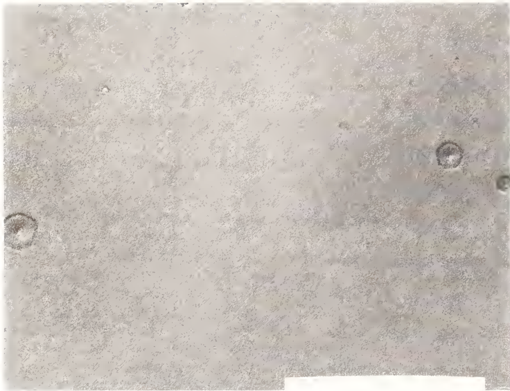
a. Single 14.5 \text{ J/cm}^2 pulse on the quarter wave thorium fluoride coating. Bar is 50 \mu\text{m} .
