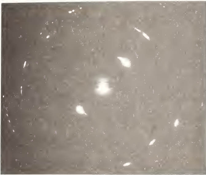
Figure 4. Selected area diffraction pattern of the subsurface deformed region of the -5 deg surface showing 29 deg of rotational misalignment.
