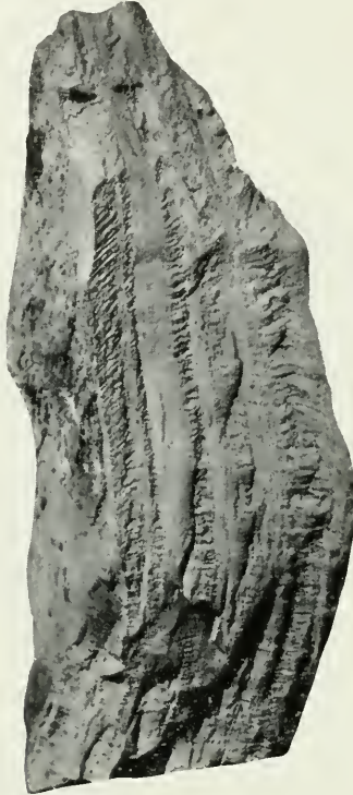
Specimen of Timiskaming sediments (natural size) from Manitou stretch, showing the relation of fracture cleavage (oblique) to bedding (vertical). This structure was developed by differential movement between beds during the folding of the sediments.
