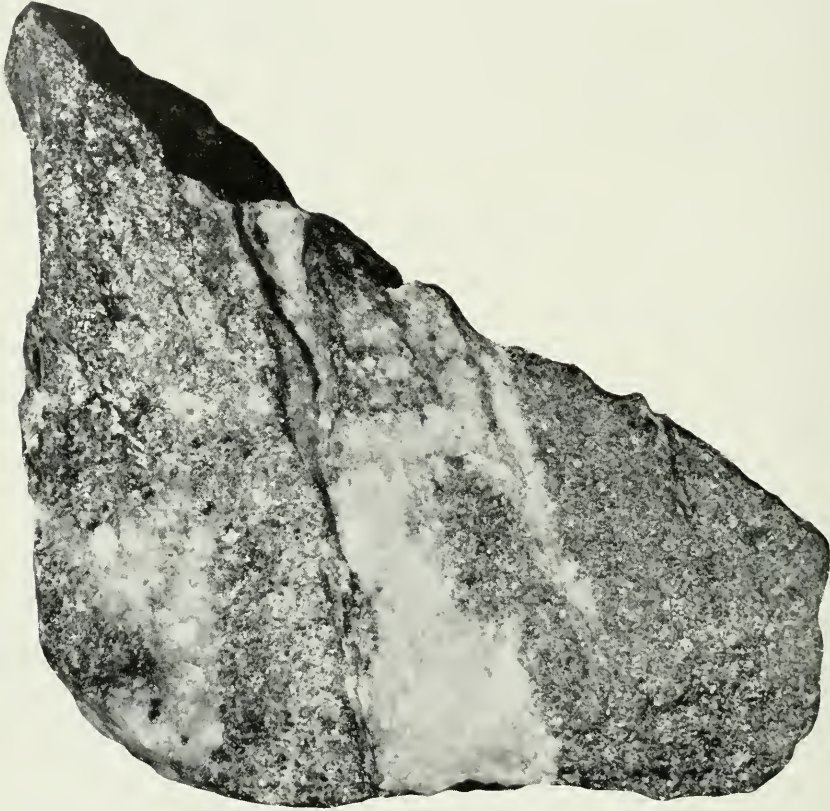
Specimen of typical gold-bearing vein material (one-half natural size) from the Konigson shaft, Straw lake. The quartz (white) is heavily mineralized with pyrite. This particular sample assayed 2.65 ounces of gold per ton.
