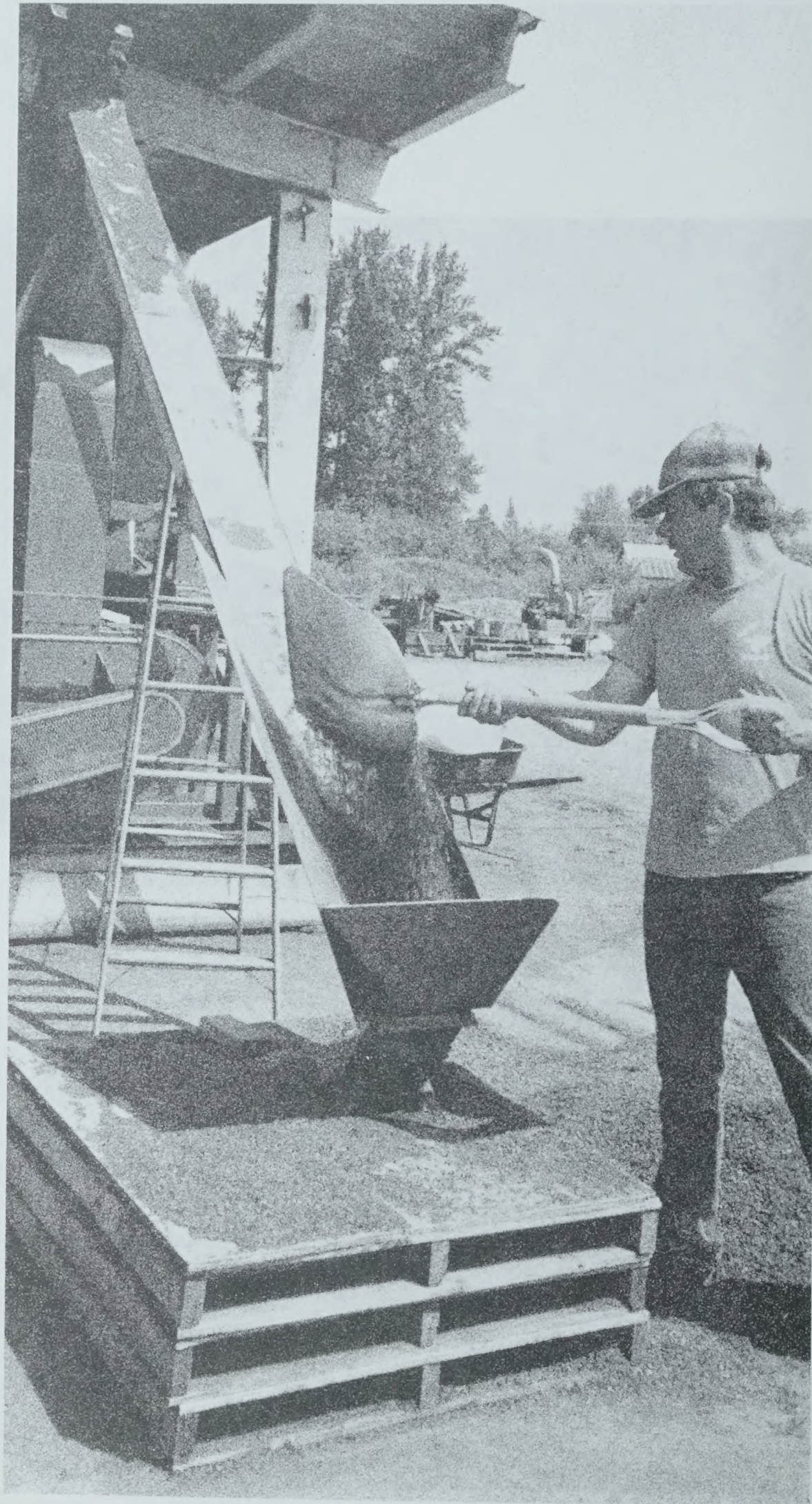
A worker loads ground bark onto a conveyor belt leading to the dryer
