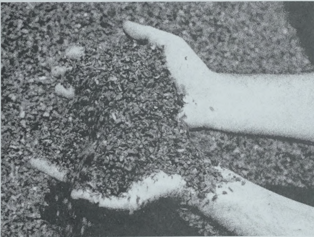
Bark ground to a uniform size, ready for drying
