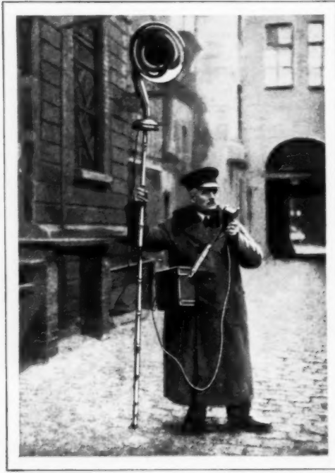
Policeman Using Portable Radio Loud-Speaker Set for Giving Orders; the Pole Is Collapsible
