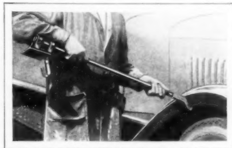
Removing Kinks in Fender Flange with Straightener
