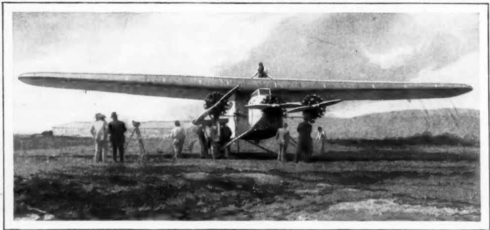
"Swinging Ship" to Adjust the Compasses by Compensating for Errors Due to the Mass of Metal in the Plane; the Picture Gives an Idea of the Typical Fokker Thick Wing
