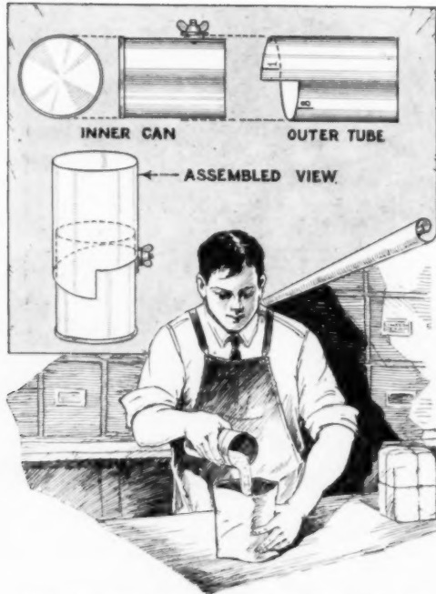
Adjustable Measuring Can for the Shop Eliminates Guessing and Weighing of Small Material
