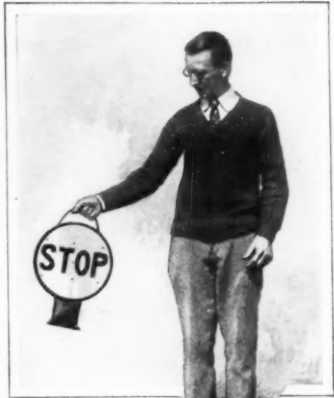
Electric Signal Lantern Made More Effective by "Stop" Warning on Red-Celluloid Disk
