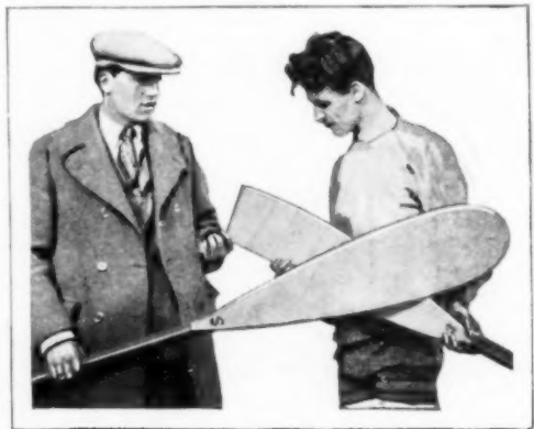
Designed for Faster Rowing; the Spoon-Shaped Oars Introduced at the University of Washington
