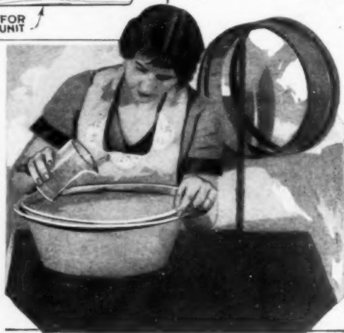
Top, Drum Dismounted Ready for Preparing the Heads; Center, Two Suitable Standard Cone Units and Detail of the Wooden Supporting Strip; Bottom, Pouring Warm Water into the Head, to Soften the Skin
