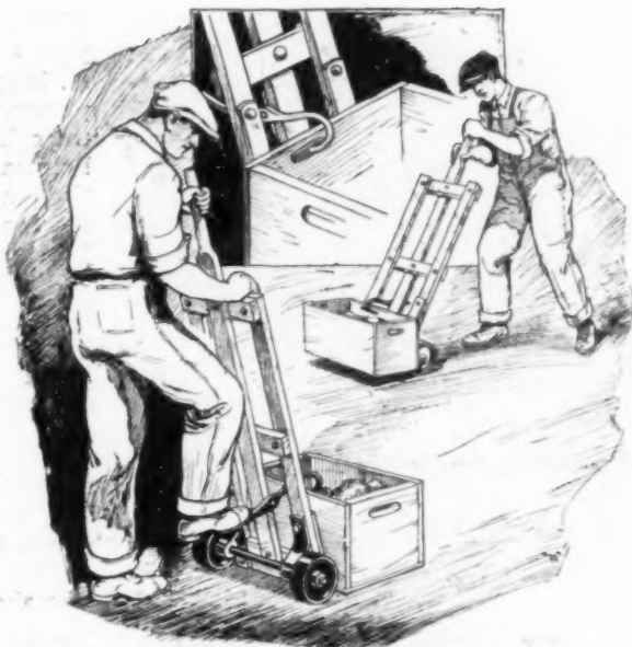
Iron Hook Pivoted to the Center Bar of a Truck Facilitates Handling Tote Boxes
