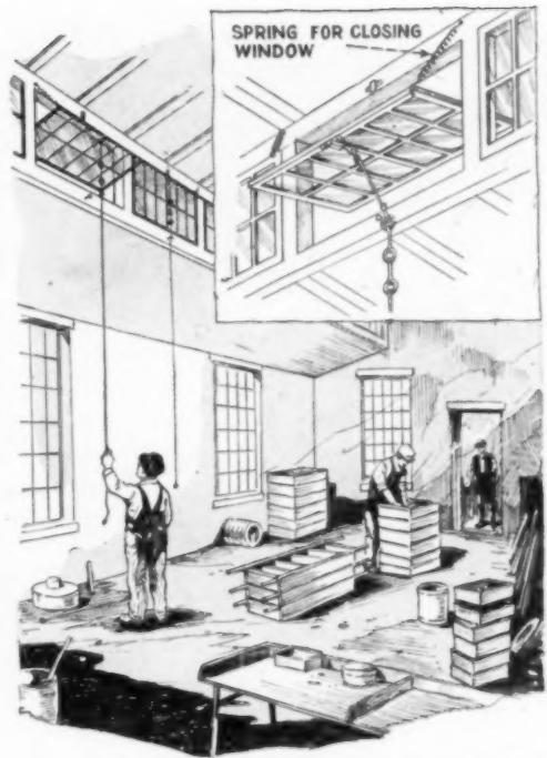
Simple Method of Opening and Holding Overhead Windows in Any Desired Position
