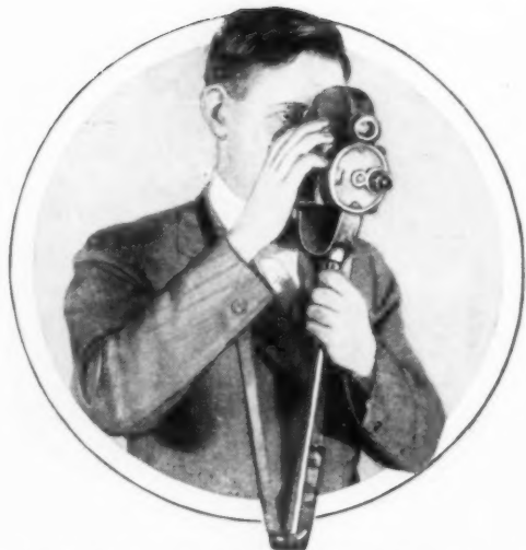
Steadying the Small Motion-Picture Camera with the Shoulder Strap and Supporting Rod
