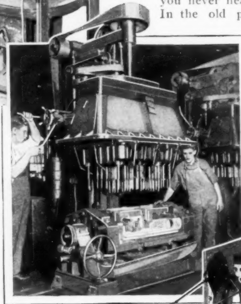
Machines That Almost Think Are Not Unusual; Above Is a Sorting Machine for Statistical Records, Designed by John K. Gore, Vice President and Actuary of the Prudential Insurance Company; in the Center Is a Gang Drill That Drills an Entire Cylinder Block in One Operation
