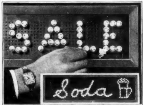
Inserting the Small Bulbs in Board, and a Sample of Illuminated Design
