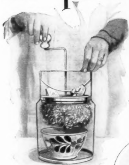
Food Press Is Easily Taken Apart for Thorough Cleaning and Has an Efficient Dasher
