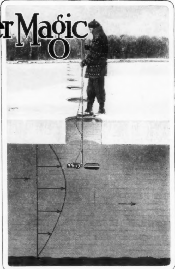
Measuring the Current Flow of a River with a Meter Lowered through Rows of Holes Cut in the Ice
