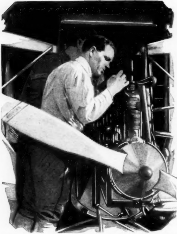
Hinkler at Work on the Thirty-Horsepower Cirrus Engine, Which Had Already Flown Vast Distances
