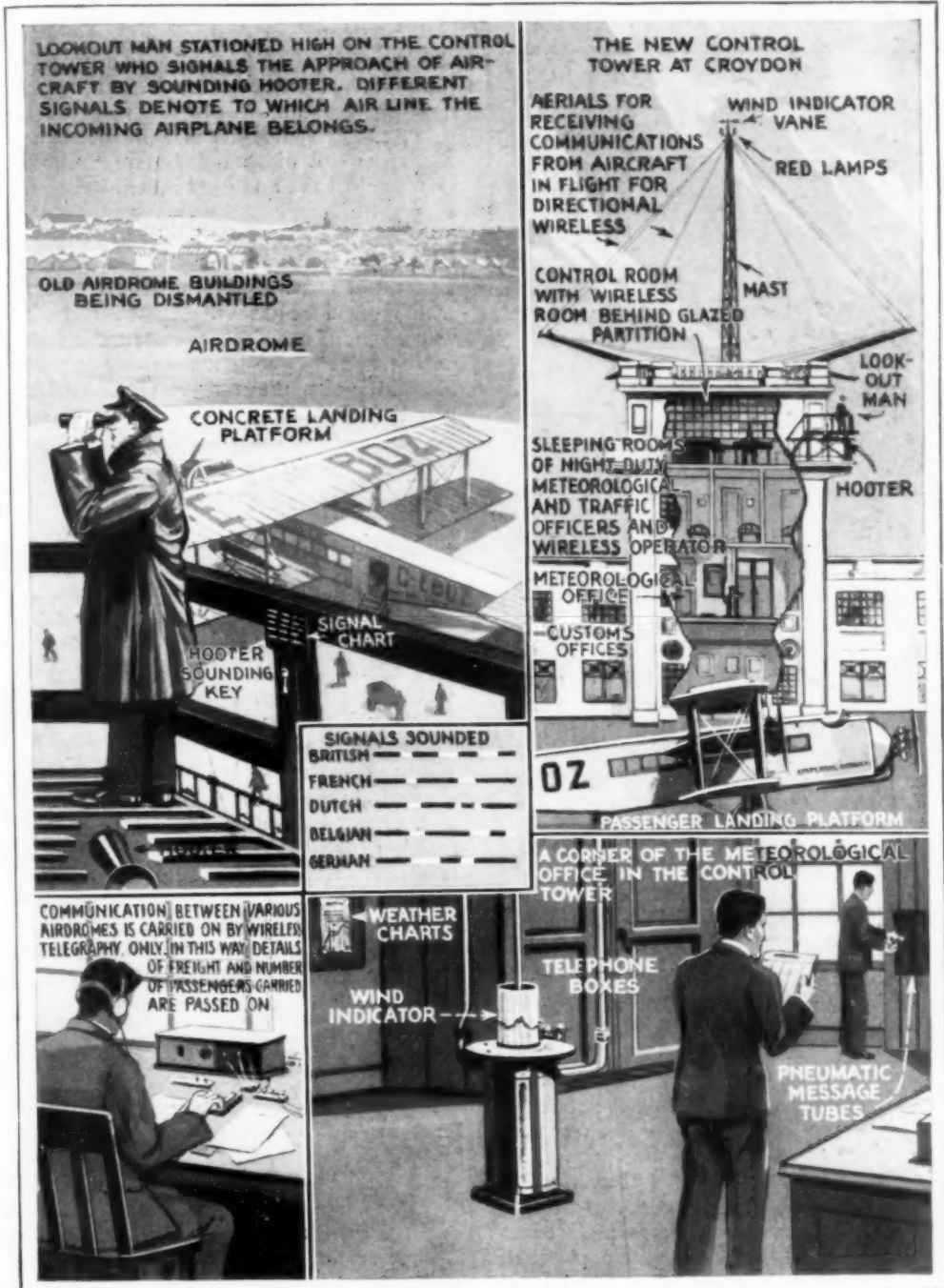
The Cross Section of the Control Tower Shows the Operating Side of the Big Airdrome from Which a Net of Air Lanes Spreads over Europe; a Horn, Called a "Hooter" in England, Signals the Nationality of Planes Sighted on the Far Horizon
