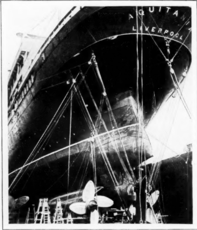
The "Aquitania" in Drydock during Change of Rudder, Which Is Seen Connected to Tackle on Ship's Sides
