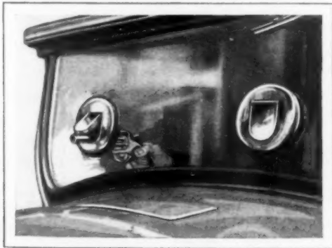
Portholes in Windshield of Police Automobile Aid in Bandit Warfare; and the Glass Is Bullet-Proof
