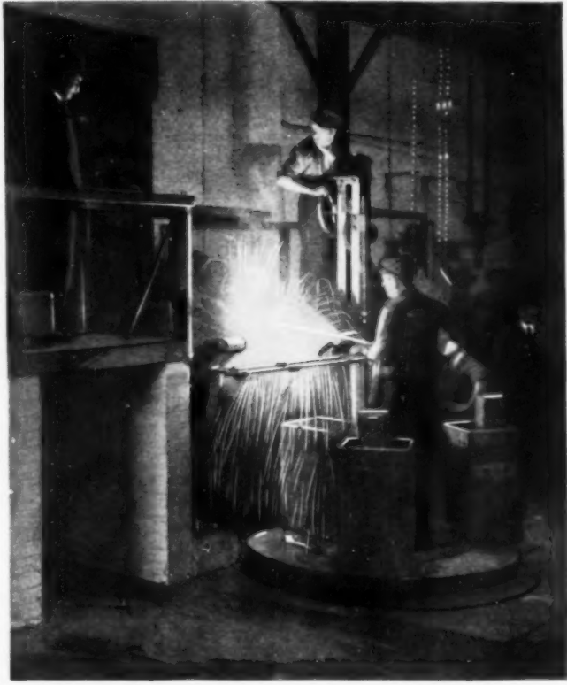
Making Crucible Tool Steel in a Wooden Box, Which Contains the Crucible and the Electric Heating Element
