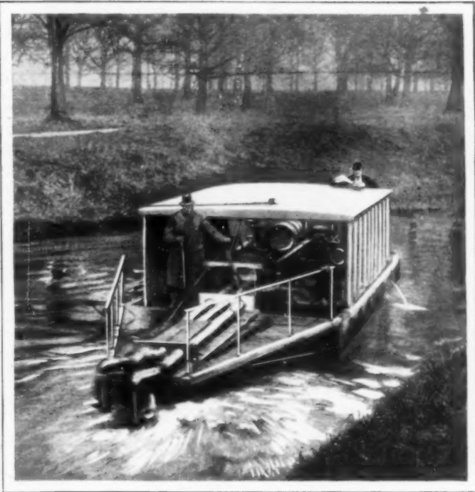
Tri-Motored Sweeping Outfit Removing Mud from the Bottom of the River Avon in New Zealand; Silt Is Stirred Up and Carried Away
