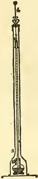
FREEZING APPARATUS WITH THERMOMETER. Fig. 95.
