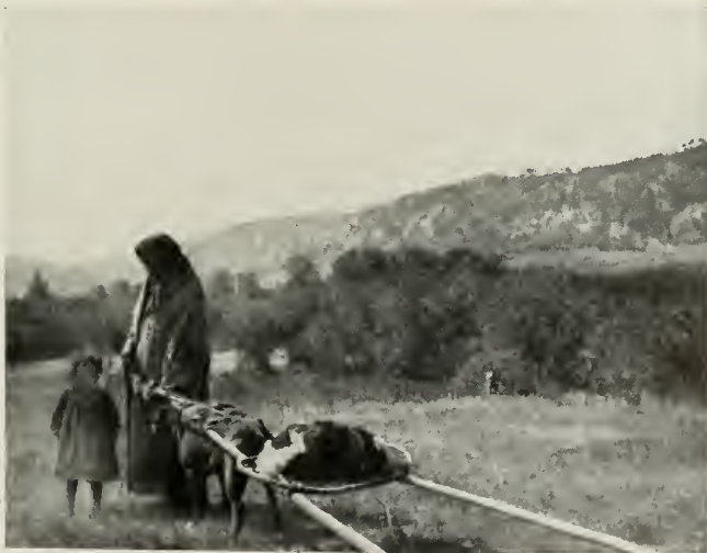
Before they had horses the Indians used dogs, attaching them to the travois, a primitive vehicle consisting of two trailing poles bearing a net or cross bar for a load. The horses of the Spaniards no doubt seemed to the Indians very wonderful "dogs"; Indian names for a horse are derived from their words for dog
