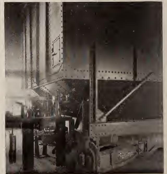
SCALE FLOOR IN PARRISH-HEIMBECKER PLANT Showing All Working Parts of Scale Above Floor Level
