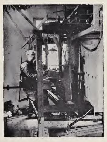
Jacquard Wearing on a Hand Loom. The loom with fly-shuttle and drop-box.
