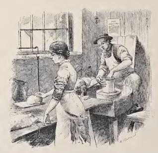
A Thrower at work. The girl weighs out the clay and supplies the potter. The wooden gauge is used to keep the size of the pots uniform.
