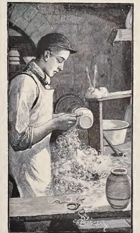
Turning pottery in the clay state on a lathe to thin down the vessels as they come from the thrower, and give them a good surface.
