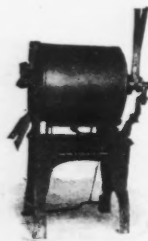
ROTARY MATRIX DRIER Heated by gas
