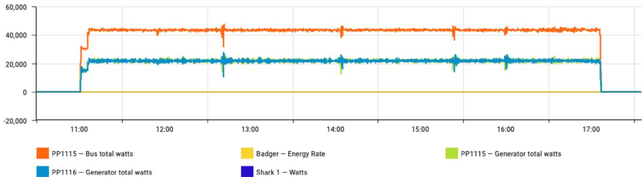
**Test on 7/15/22 ran over 6 hours, with combined power generation at 43 kW. Periodic power variation during feedstock refilling events.**
