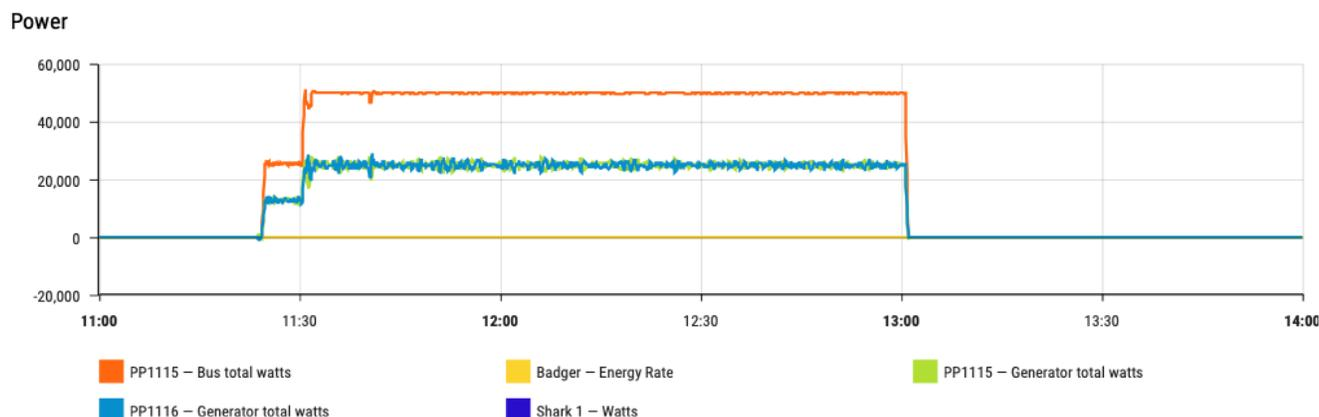
**Test on 7/14/22 operating at 72 Hz yielded a combined power output above 50 kW.**
