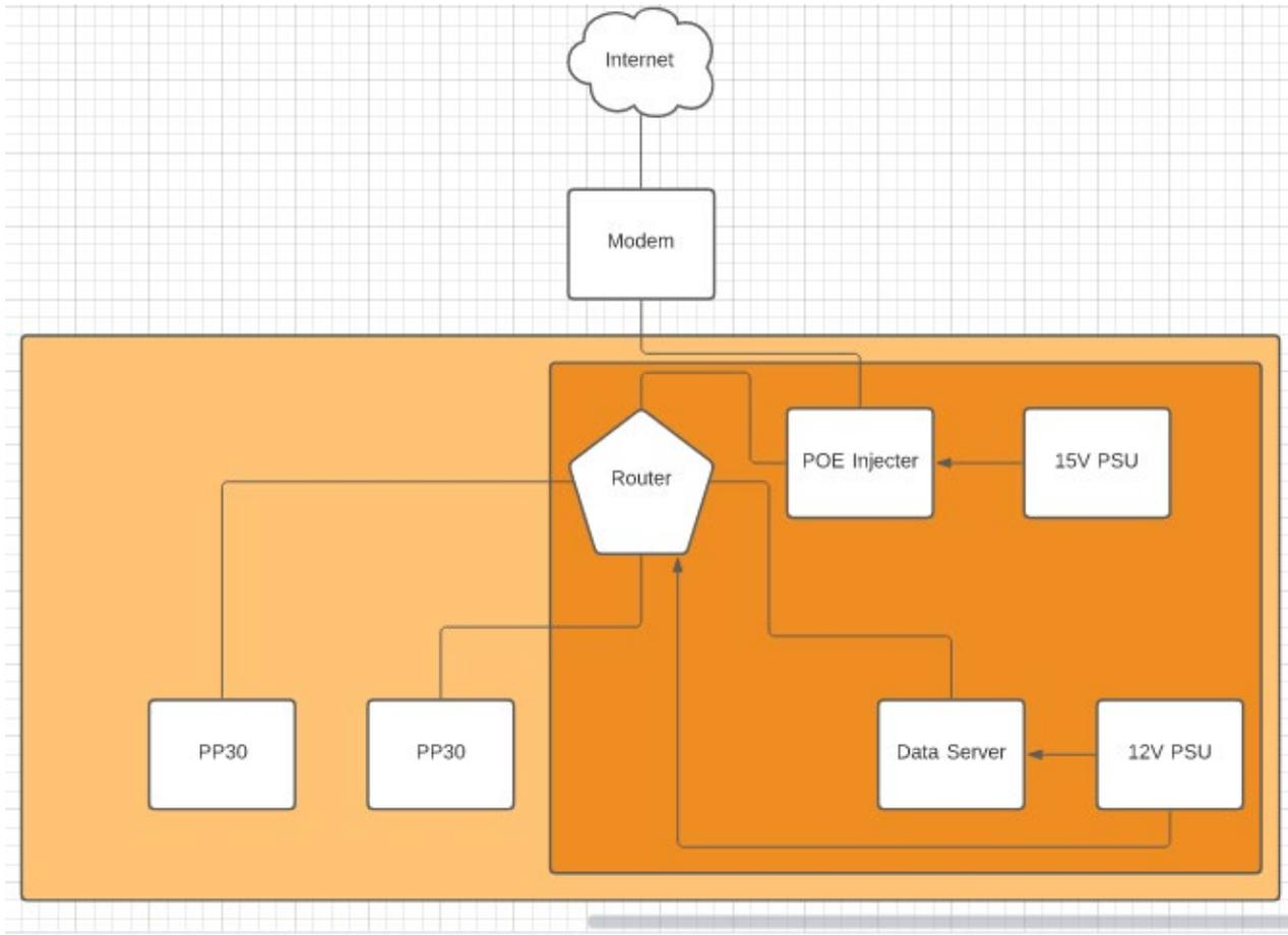
**Container: light orange; Remote Monitoring Enclosure: dark orange (not to scale)**
