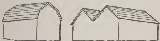
Curb Roof. M-Roof.
