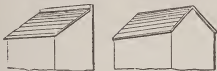
Shed Roof. Gable Roof.
