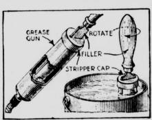
Cheaply Made Filler Saves Time in Charging a Pressure Gun With
