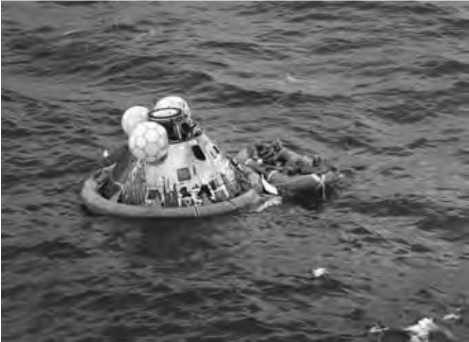
Figure 4.1 Flotation collar attached to the Columbia Command Module. The three astronauts plus a Navy swimmer sit in the recovery raft, awaiting pickup by helicopter. All four men are wearing BIGs.
