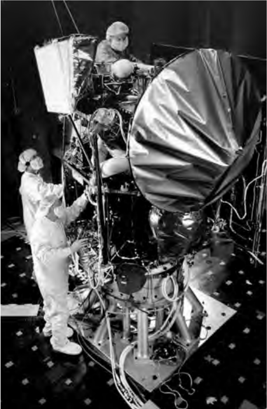
Figure 7.1 Assembly of MCO.
