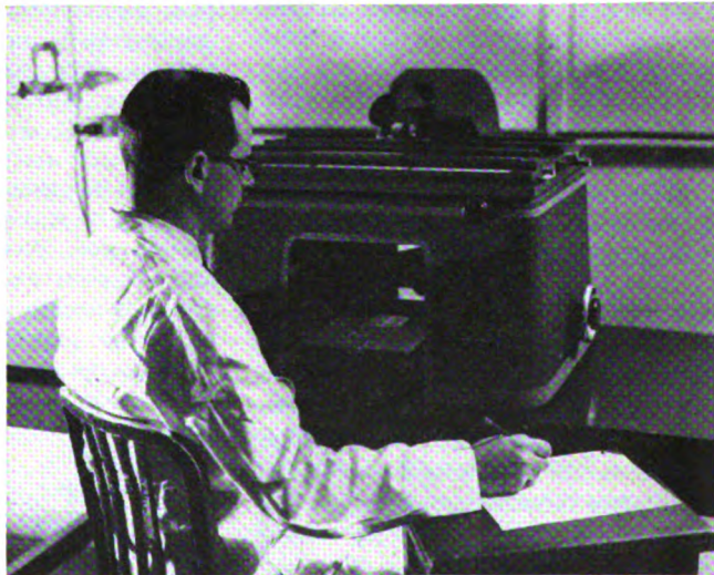
and prevention of room contamination. Figure 2—A comparator-densitometer, Jarrell-Ash model 200. The spectrographer is matching standard and sample spectrograms in the semiquantitative determination of metals. He was able to complete as many as 1500 determinations a day.
