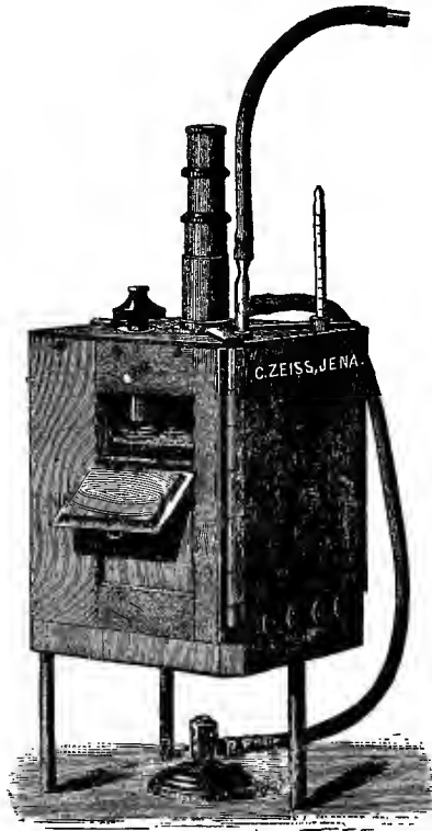
Method of enclosing a microscope within a warm box
