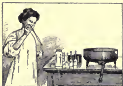
FIG. 176. Putting the milk into the test bottle. The pipette is held at an angle with the test bottle and its point against the inside of the neck.
