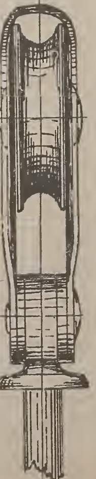
LIGHT SHEET METAL, DECK-LEAD BLOCK, PATENTED SHEEVE.
