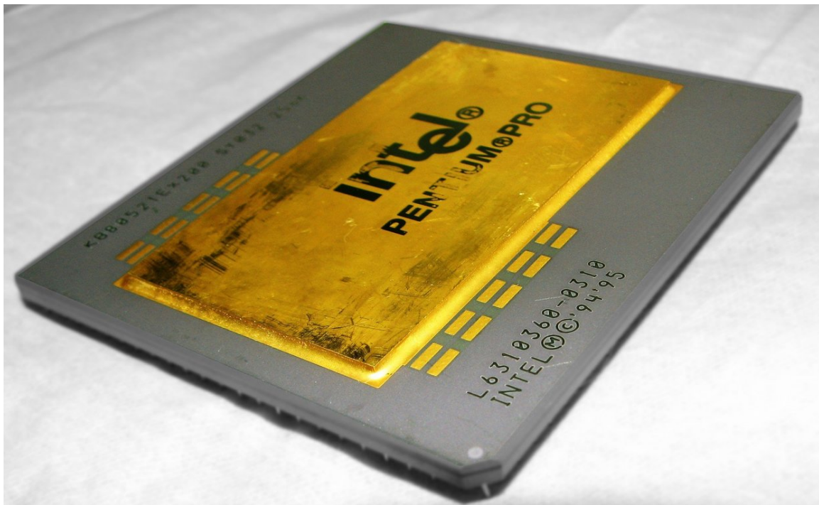
Figure 71 The Pentium Pro chip was one of the largest microprocessors ever manufactured. It was so large because it contained the largest cache of any chip at the time.
