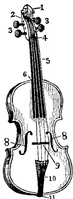
【Violin ① (Stradivarius)】 1 Scroll; 2 Peg Box; 3, 3 Pegs; 4 Nut; 5 Finger board; 6 Neck Plate; 7, 7 Bouts; 8, 8 Sound Holes; 9 Bridge; 10 Tail-piece; 11 Button.
