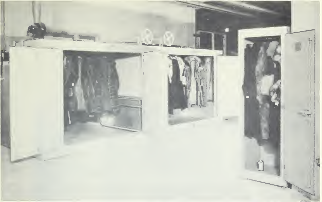
Figure 1.--Two types of metal vaults such as can be purchased or built according to space and commodity need. These vaults are used for treating the day's arrival of fur coats offered for summer storage. After an overnight fumigation in these vaults the furs are removed to large permanent storage vaults. (Figure 24 of Cir. 369.)
