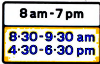
Fig. 25b. Plate showing (above) hours during which waiting is prohibited and (below) hours during which loading and unloading are prohibited. (Paragraph 85.)
