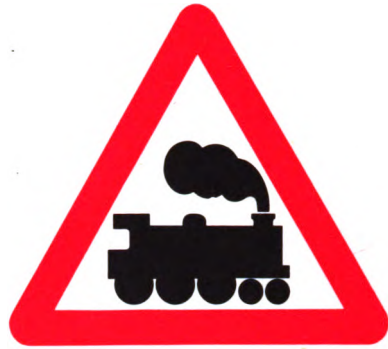
Fig. 49. Level crossing without gate or barrier. (Paragraph 101.)
