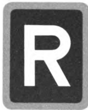
Fig. 96. Ring road repeater sign. (Paragraph 155.)
