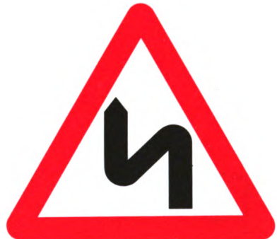
Fig. 38. Double bend, the first to the left. (Paragraph 91.) (The symbol may be reversed.)
