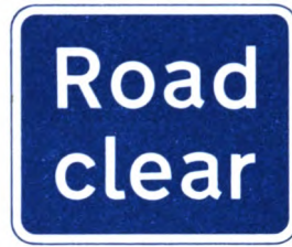
Fig. 141. End of temporary obstruction. (Paragraph 194.)
