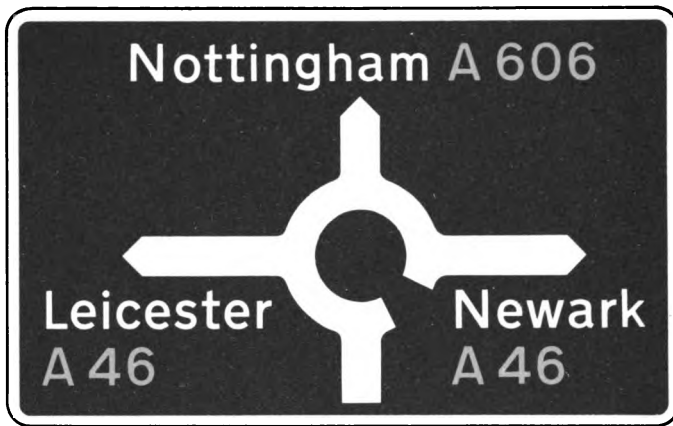
Fig. 80. Advance direction sign for roundabout junction. (Paragraph 148.)
