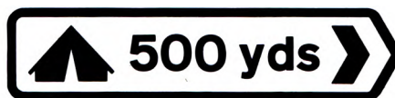
Fig. 128. Direction and distance to camping site (tents). The symbol may be varied as appropriate. (Paragraph 190.)
