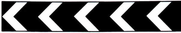
Fig. 40. Sharp deviation of route to the left, for use on roundabouts and at dangerous bends. (Paragraph 110.) (The chevrons may be reversed according to direction.)
