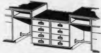
Depressed counter top assembly for teller's machine.
