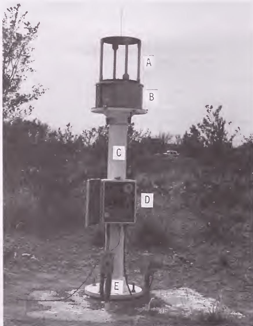
Figure 2. Lightning Location and Protection, Inc. Model 141 Advanced Lightning Direction Finder located at Socorro, NM. Components include antenna assembly (a); electronic module with three circuit boards (b); mast (c); AC power supply (d); and communication and power cables (e). It is part of the national network of wideband magnetic direction finders, an accurate system for lightning detection.
