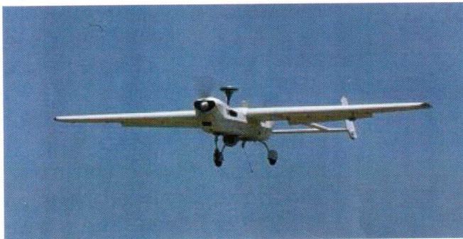
Imagery Intelligence is i.e. provided by the „Unmanned Aerial Vehicle“ (UAV) HUNTER for a detailed real-time picture of an ongoing situation.
