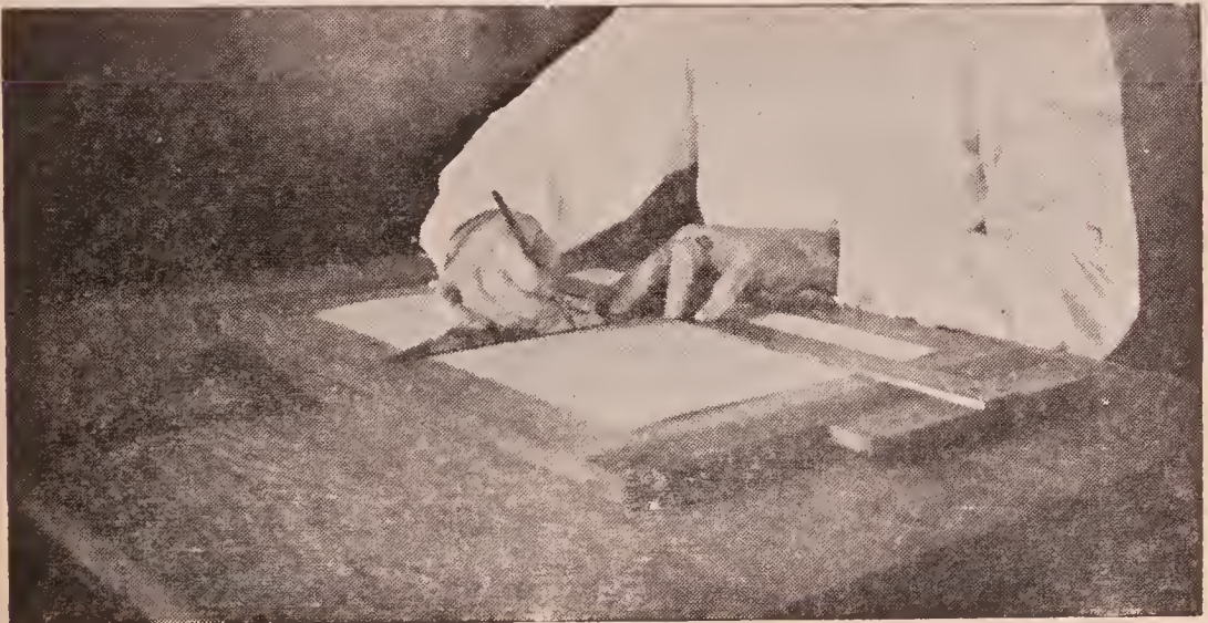
Fig. 61. Inking vertical lines with ruling pen.
