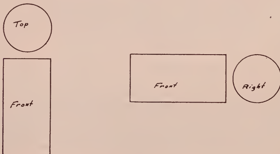
Fig. 51. Two views of a cylinder shown in two positions.
