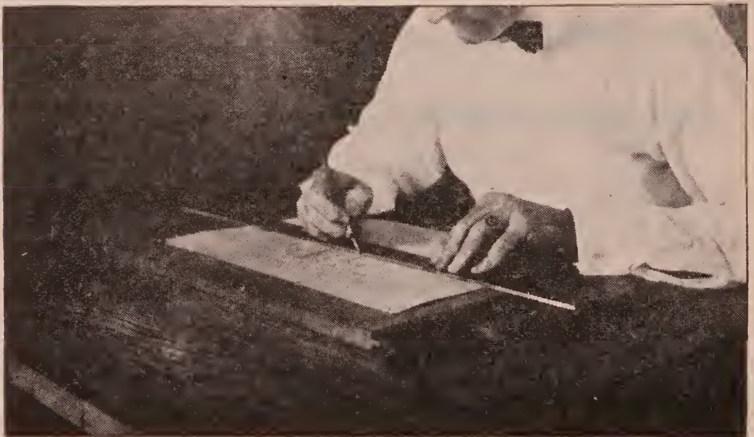
Fig. 60. Inking horizontal lines with ruling pen.
