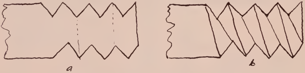
Fig. 115. Sketching a single-thread sharp "V" screw.
