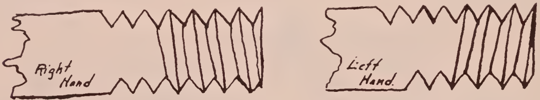
Fig. 118. A right hand and a left hand thread.
