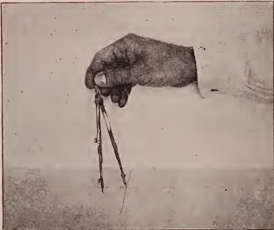
Fig. 62. The position of compass and hand when inking a circle.
