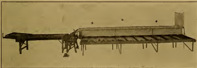
Fig. 24.—A GRADING MACHINE
