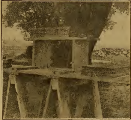
Fig. 33.—A FORM FOR SETTING UP APPLE BOXES
