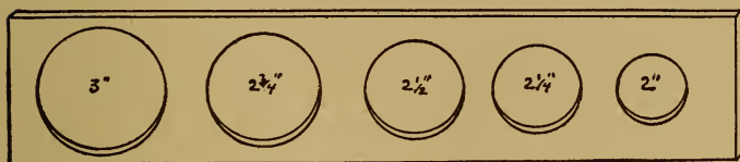
Fig. 22.—SIZING BOARD, 18" x 4" x \frac{3}{8} ".
