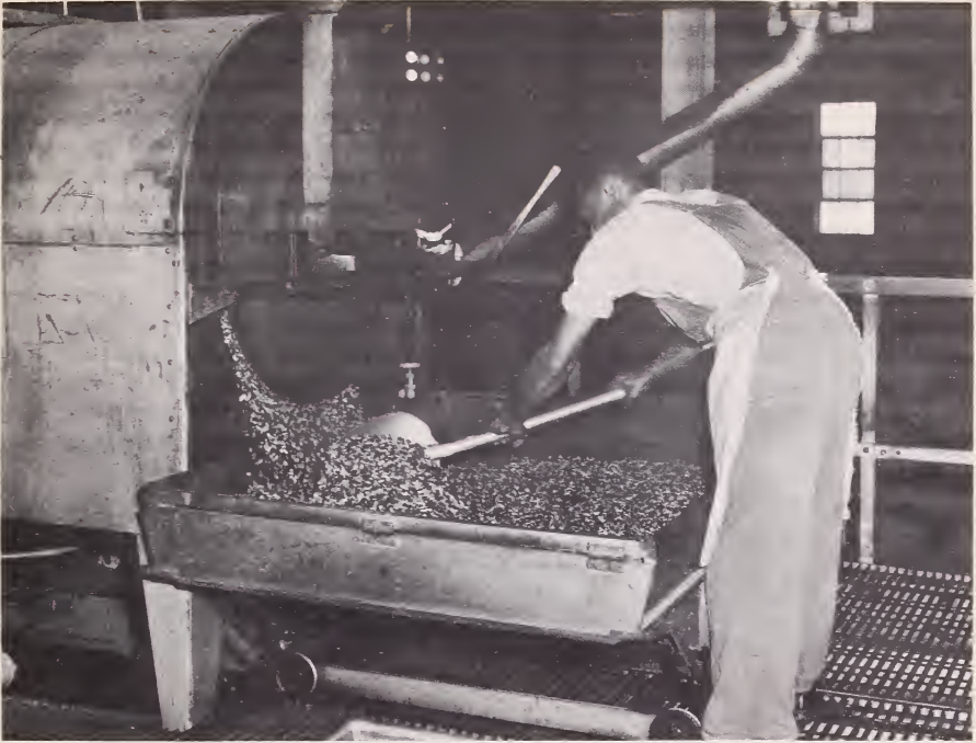
FIGURE 18.—Roasted Runner peanuts being dumped from roaster into cooling trays.
