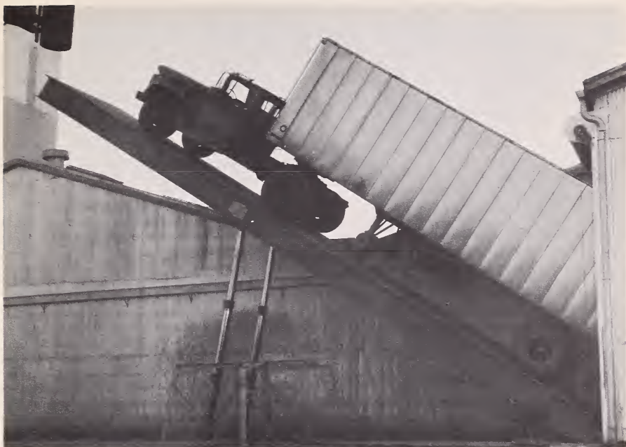
FIGURE 7.—Unloading a truck of bulk peanuts at a sheller's plant required only a few minutes with this hydraulic dumper.
