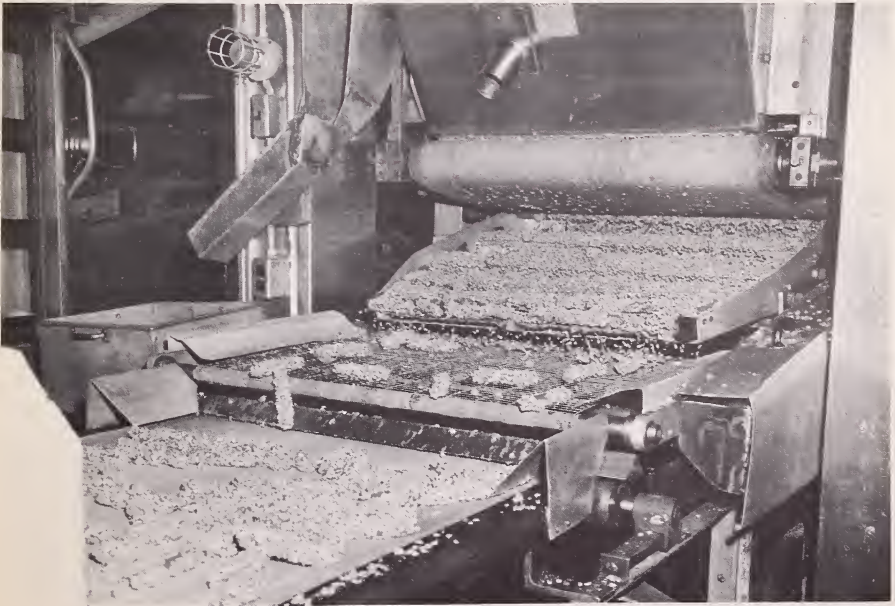
FIGURE 29.—Machine which enrobes the centers for chocolate "nut rolls" with hot caramel and then coats them with peanuts. The peanuts are being added from the hopper on the upper right of the picture.
