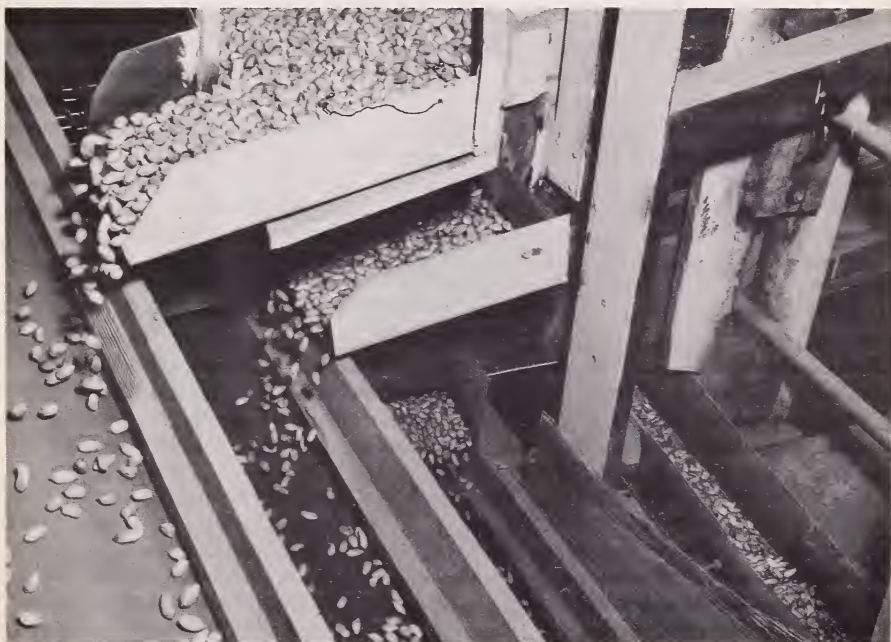
FIGURE 16.—The discharge spouts of a sizing machine. This is the final step before the shelled kernels are bagged.
