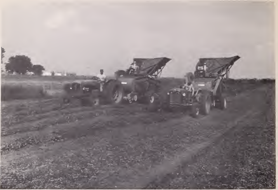
FIGURE 3.—Combine-pickers in operation in the Southeast. The peanuts are elevated to the hoppers. When the hoppers are full, they are dumped into a truck for delivery to an artificial drying plant or to a cleaner and sheller.
