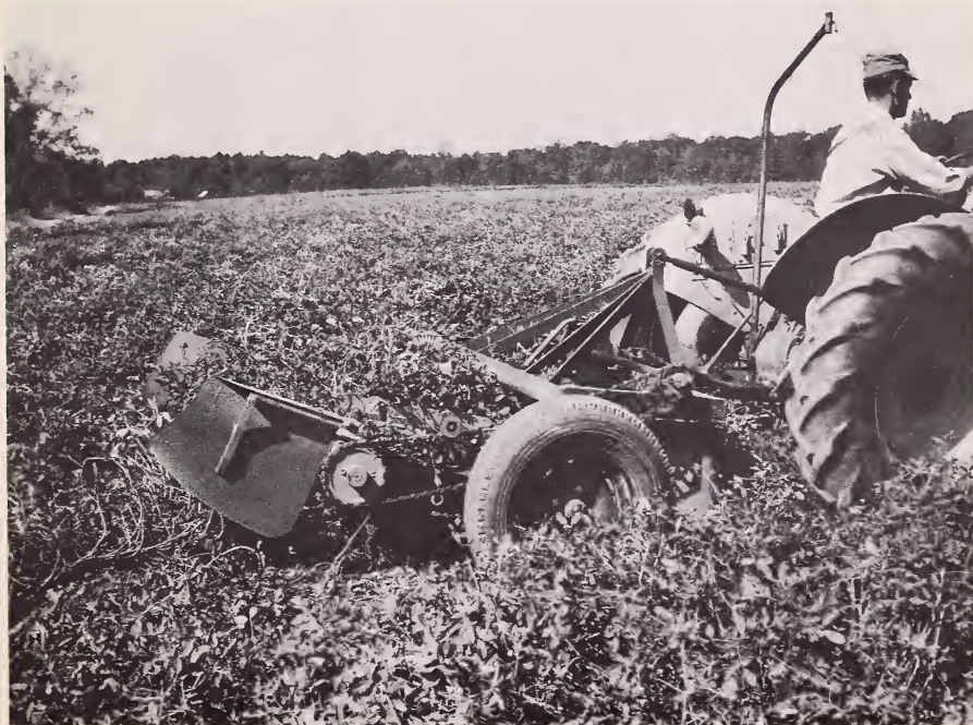
FIGURE 2.—Peanut digger in operation.
