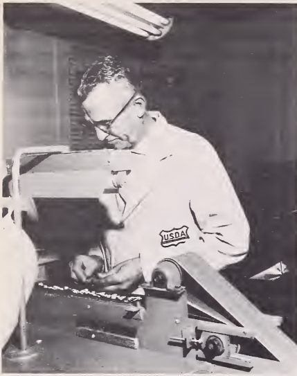
FIGURE 11.— Federal-State inspector examining sample of split peanut kernels coming out of mechanical splitter used by Federal-State Inspection Service as part of official grading procedure.
