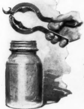
For Opening Fruit Jars and Other Containers, This Efficient Wrench Is Adapted to Different Sizes and, on the End, Has a Bottle Opener; Wrench Is Constructed to Hold the Cover Firmly
