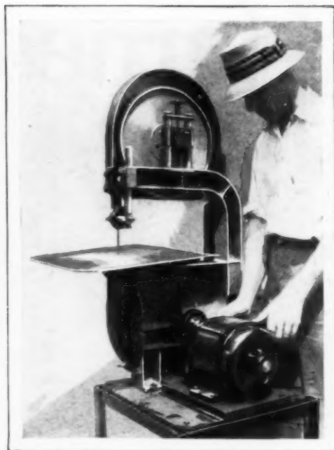
Portable Bandsaw Outfit Ready for Use; It Weighs But 135 Pounds and Is Easily Moved About
