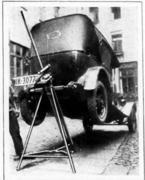
Portable Jack in Use; Raising Is Done with a Crank and Worm; Car Can Be Lifted to Steep Angle
