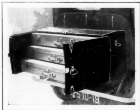
Auto Luggage Carrier Open, to Show the Suitcase Drawers That May Be Removed and Used Separately
