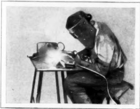
Hydrogen Welding Outfit Which Can Be Used on Many Alloys and Thin Sheets
