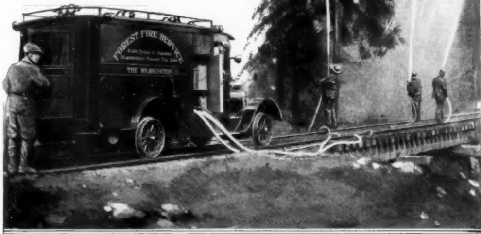
Forest Rangers Testing a New Rail Motor Car, Equipped to Fight Forest Fires in the Virgin Timber of Washington; the Powerful Pumps Draw the Water from the Nearest Stream
