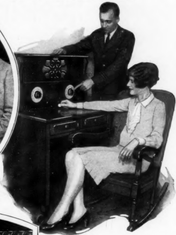
James Cantwell Instructing Miss Edith Nelson How to Operate the New Coin-in-the-Slot Radio Receivers Recently Installed in the Hotel Sherman, Chicago; the Instrument Is Designed to Operate Thirty Minutes for Each Quarter Deposited; after Dropping the Coin, the Set May Be Tuned to Any Station Desired
