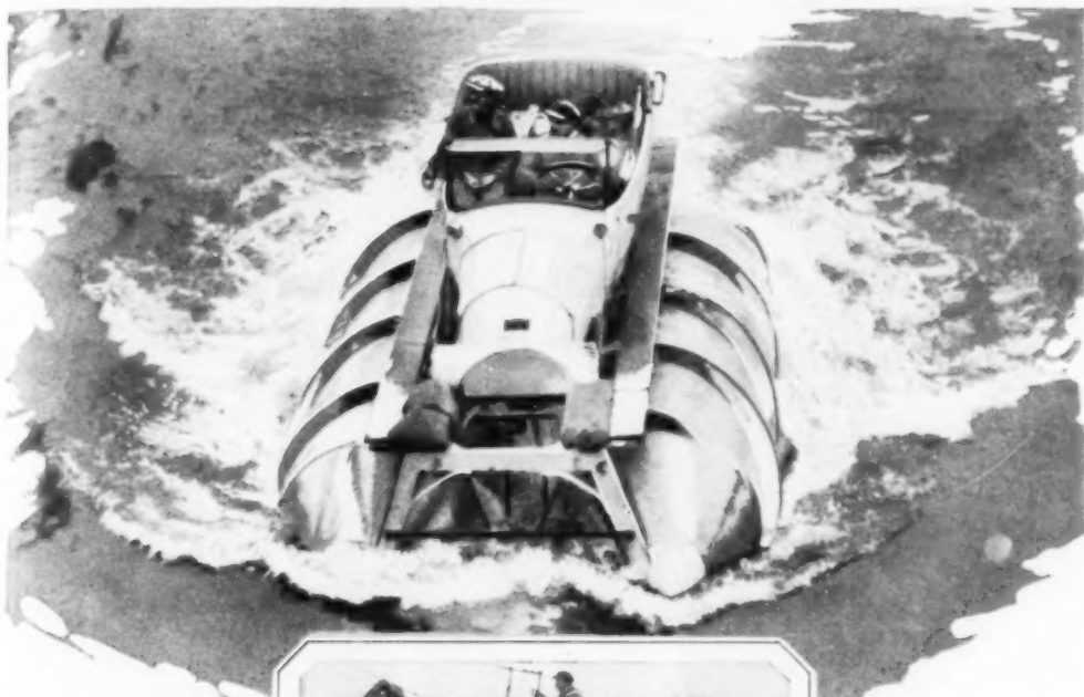
Boat in Action and a Side View, to Show the Construction of the Revolving "Propeller Tube"
