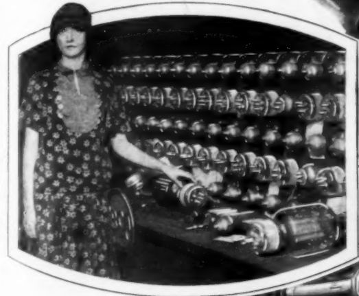
Above, Transmitting Tubes Ready for Final Factory Tests; These Tubes Are Somewhat Larger Than the Familiar Receiving Tubes as Demonstrated by the Comparative Size of the Young Lady Shown in the Photo; Right, Comm. G. M. Dyott's Radio Apparatus, Including Dry-Battery-Powered Transmitter, in Use on His River of Doubt Expedition; Similar Equipment Will Be Carried on His Patagonia-Panama Exploration Trip
