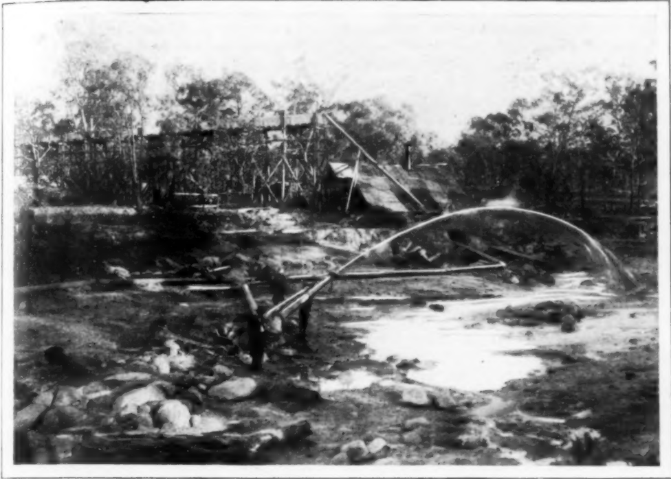
Placer Mining for Tin in New Zealand; More Than Five-Sixths of the World's Tin Is Found as Rolled Lumps and Grains in Alluvial Gravels, from Which It Can Be Washed
