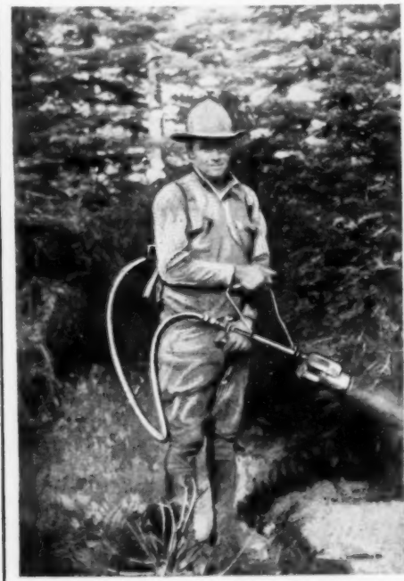
To Speed the Starting of Backfires; Blow Gun That Shoots Gasoline on Forest Brush
