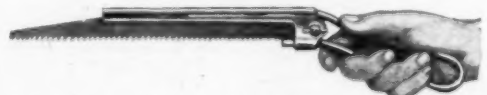
Saw Blade Fitted in Holder Which Is Adapted to the Further Use of Broken Pieces
