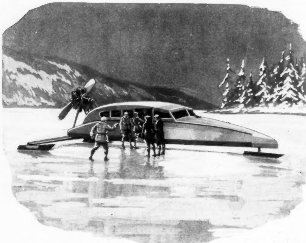
Aided by a Strong, Favorable Wind, Propeller Iceboat of This Type Has Reached a Speed of Nearly 150 Miles an Hour; the Passenger Compartment Is Comfortably Furnished
