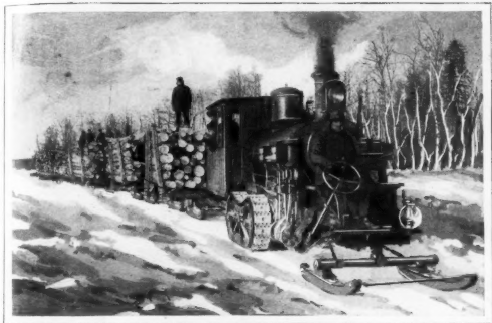
Steam Locomotive Mounted on Endless Treads, with a Pilot Sled Steered by a Gear Operated from the Front of the Boiler, as Used in the Minnesota Woods
