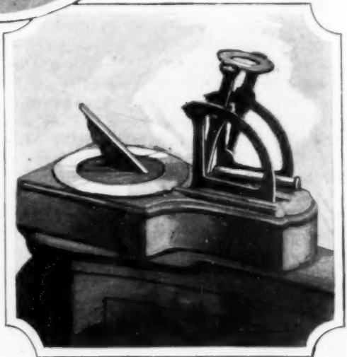
Two Sun Furnaces and, Below, a Sundial and Noon Gun, the Latter Being Fired by Rays Focused on the Touch Hole by a Lens
