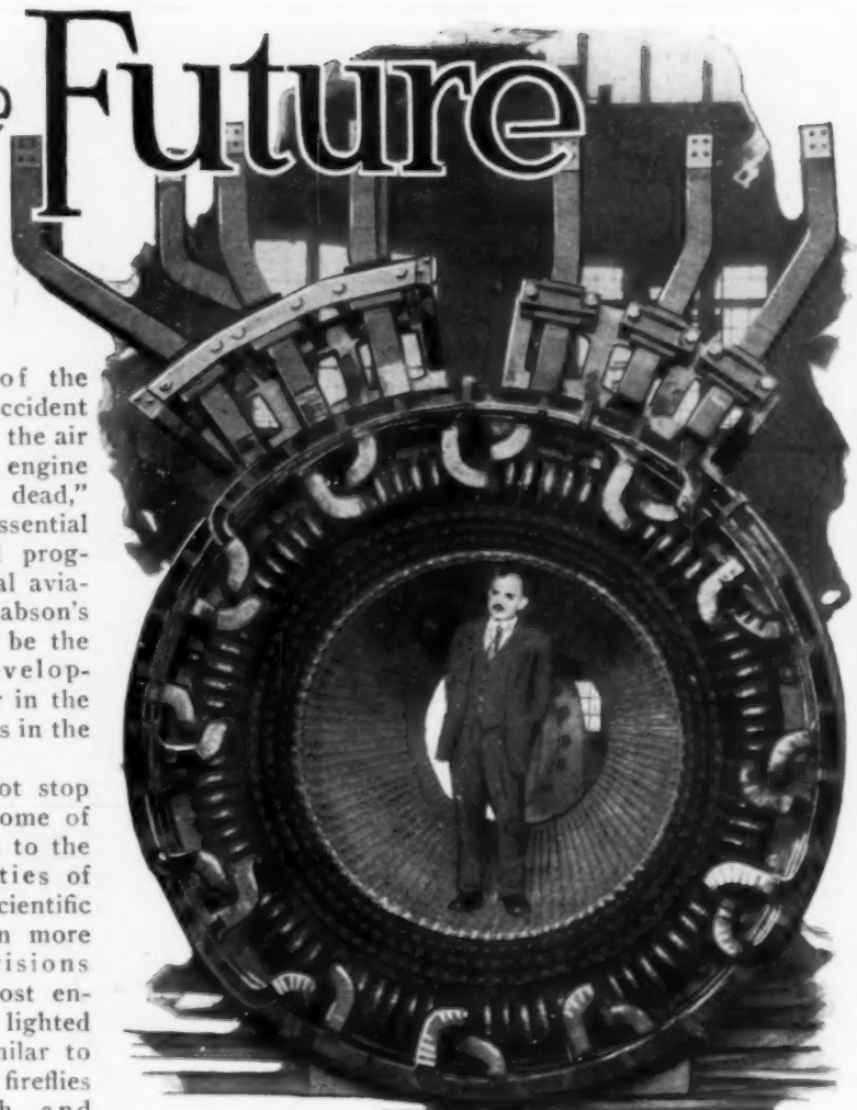
A Powerful Giant of the Electric Age; Huge Stator Winding and Connections with Supports on Inside Frame Structure
