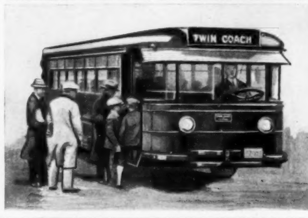
Twin Motor Bus Which Has Two Engines with Controls at Either End and Can Make High Speed with Big Loads
