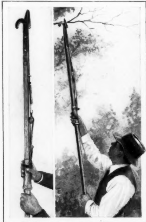
Close View of the Trimmer, Showing the Block-and-Tackle Rig and Cutter as Though in Use
