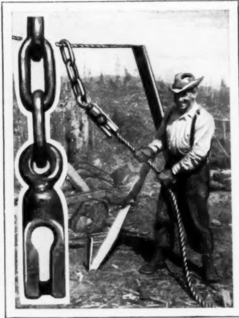
Close View of the Hook, and How Easily It Is Connected with Only a Little Slack
