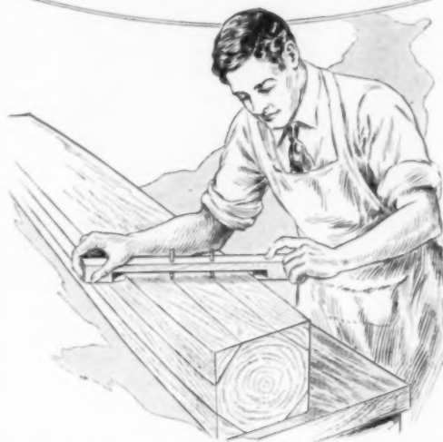
Improvised Gauge for "Eight-Squaring" Large Tapered Pieces of Timber
