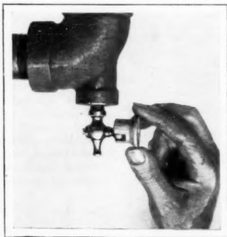
Wooden-Spool Handle for Radiator Drain Cocks
