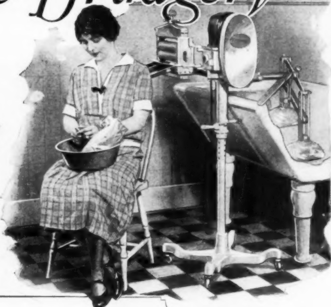
Portable Electric Unit That Makes a Washing Machine Out of the Laundry Tub; the Cups Plunge Up and Down to Remove Dirt
