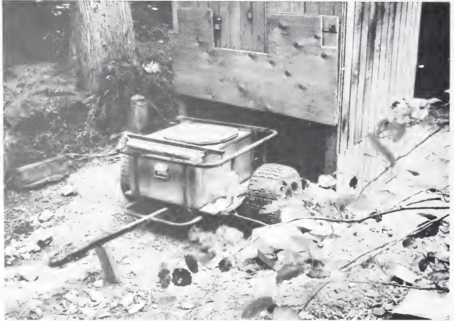
Figure 10. ATV vault with lid in place for transport.
