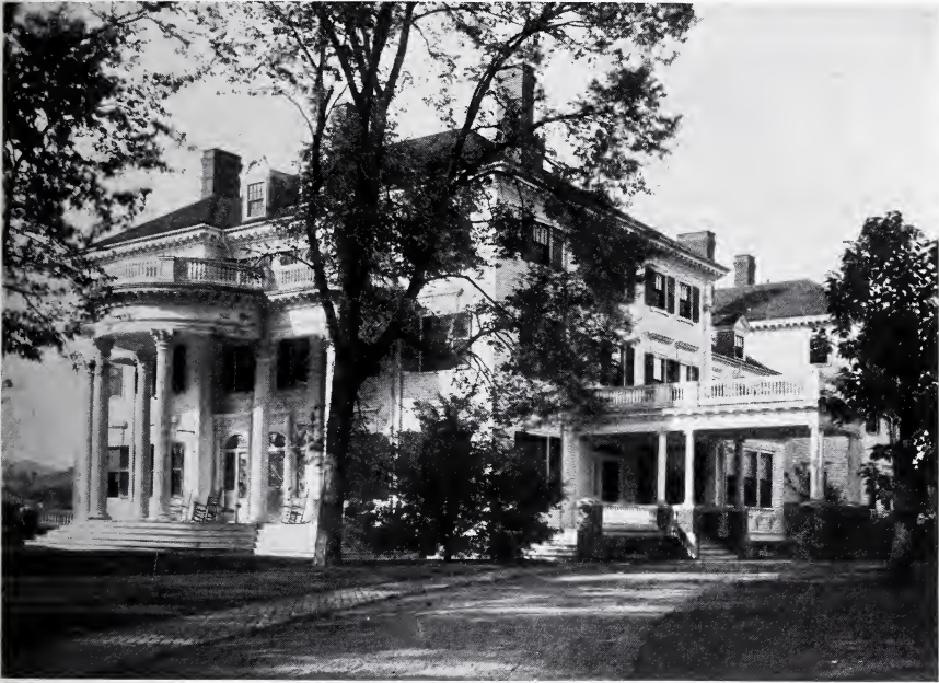
13. A college fraternity house embodying colonial adaptations of the classic. Note the Corinthian facade and the Ionic columns of the porte cochere. Photo by H. E. Kinsman.
