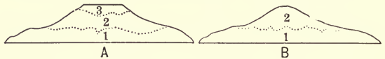
FIG. 164.—Diagram to illustrate the occurrence of residual and colluvial limestone soils on (A) a flat-topped hill and (B) a round-topped hill. (1) colluvial loams; (2) stony loams; (3) residual silt loams.
