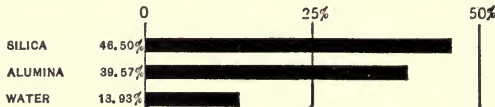
FIG. 34.—Diagram showing the composition of pure kaolinite. (After Clarke, U. S. Geological Survey.)
