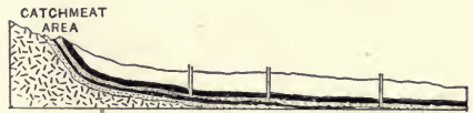
FIG. 108.—Generalized diagram showing the catchment area east of the Rocky Mountains from which the sandstones (dotted) carry the underground water beneath the Plains.
