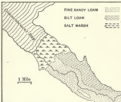
FIG. 143.—Soils of the Puyallup River delta, Oregon. The river is building its delta into Commencement Bay. (U. S. Bureau of Soils.)
