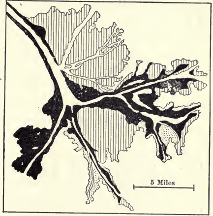
FIG. 142.—Map of the “passes” of the lower Mississippi delta showing the areas gained by deposition and those lost by wave and current erosion. The black areas show the area of the delta in 1872, the lined areas, the regions of deposition and the dotted areas, the regions eroded. (U. S. Coast and Geodetic Survey.)
