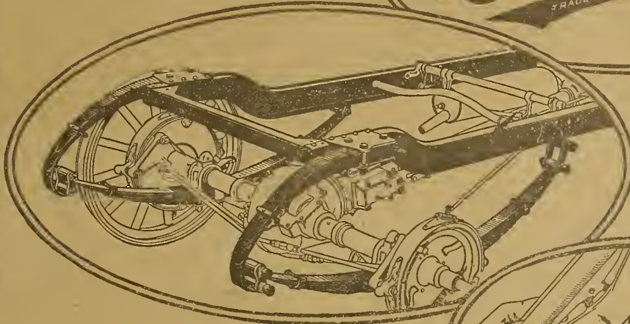
New underslung shock-absorbing rear springs
