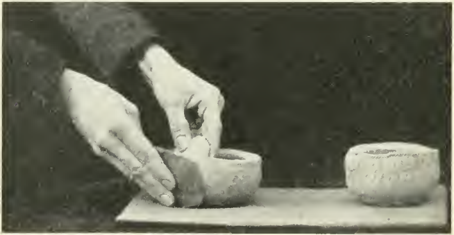
FIG. 173. Shaping with Rough Piece of Pottery.
