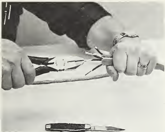
A.— Twist individual wires (three conductor cable is being used for loop).
