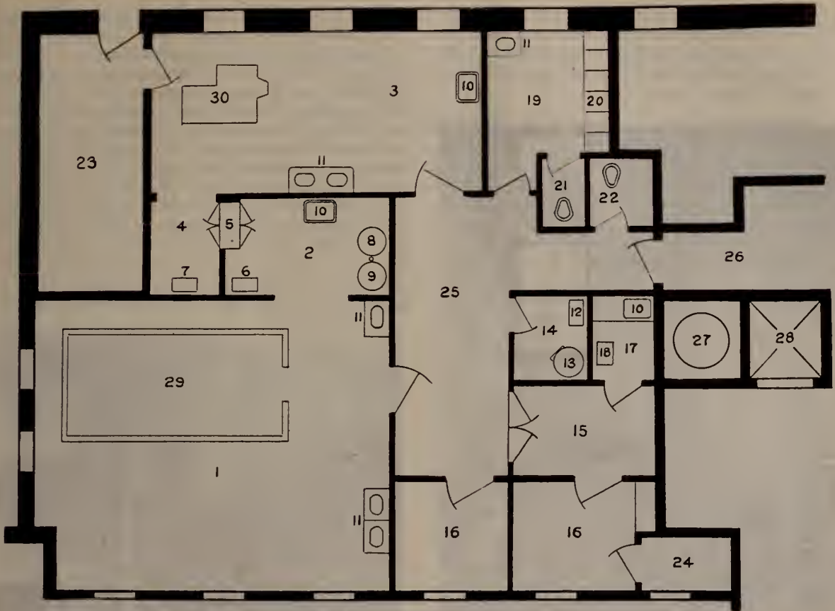
Fig. 2.—Plan View of the new operating pavilion for Thoracic surgery at the German Hospital, New York.
