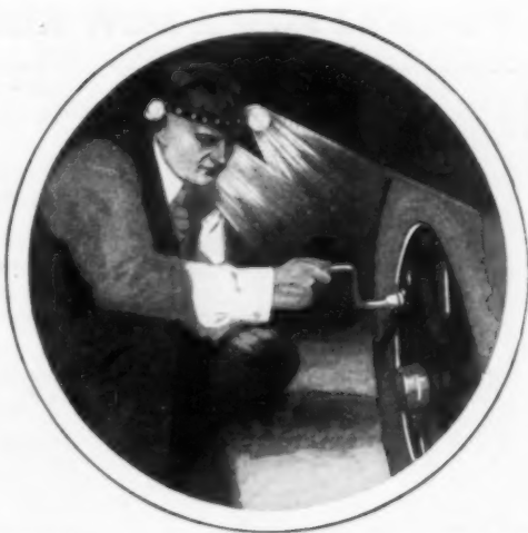
Changing Tire with Aid of Electric Lamps That Are Worn on Headband for Better Vision
