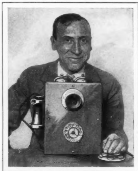
Automatic Telephone Box That Conceals a Motion-Picture Camera for Trapping Criminals
