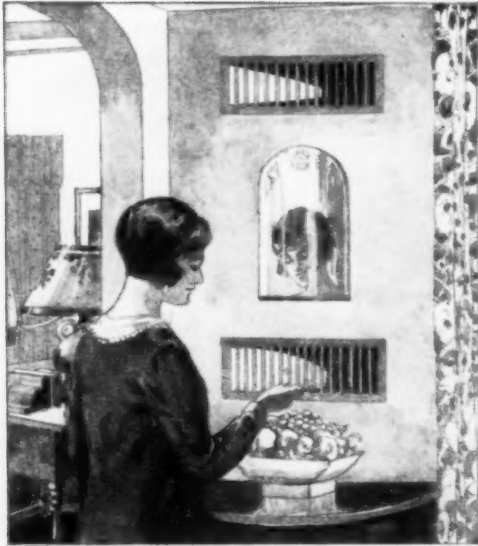
Drawing to Show Installation of the Air-Washing Cabinet; the Spray Is behind the Wall
