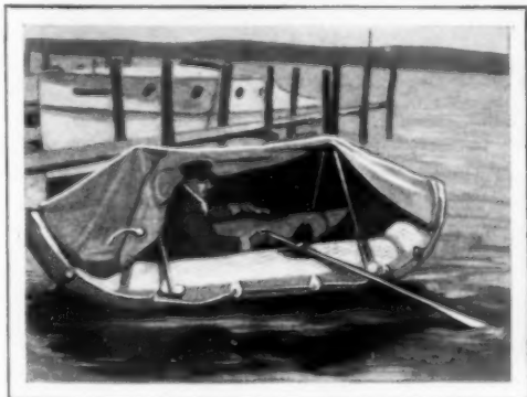
"Tire" Boat in Use; It Is of Fabric That Can Be Folded into Small Bundle When Deflated
