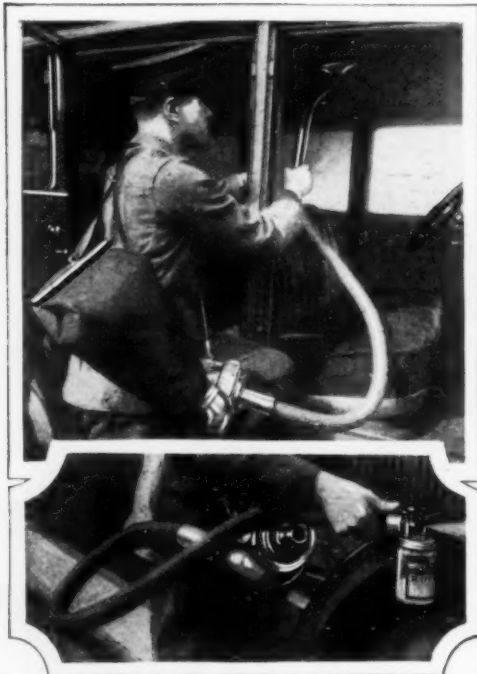
Using the Cleaner to Remove Dust from Car Interior and as a Sprayer for Painting.
