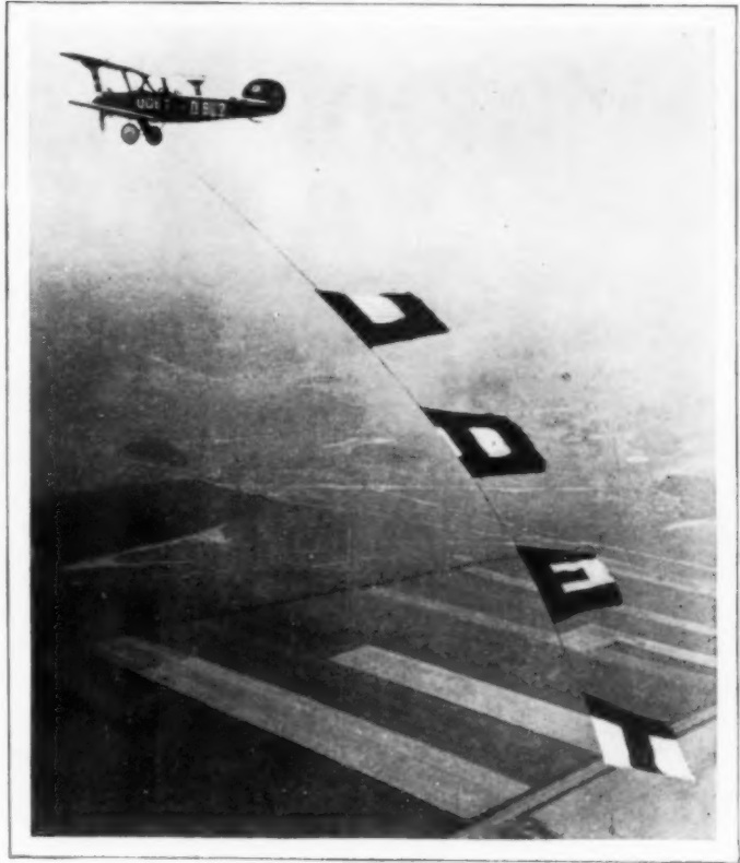
Chain of Flags Bearing Letters and Towed from Plane to Form Message Which Is Visible for Many Miles
