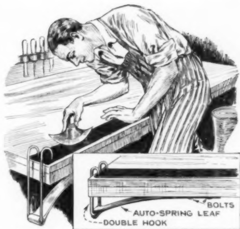
A Strong and Convenient Strap Holder Is a Timesaver for the Harness Repair Man
