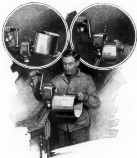
Metal-Working Unit and Three of Its Operations; Note the Inclosed Gears
