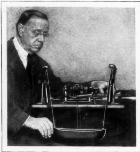
Model of the Lifeboat Which Can Be Launched in Few Seconds by Pressing a Button
