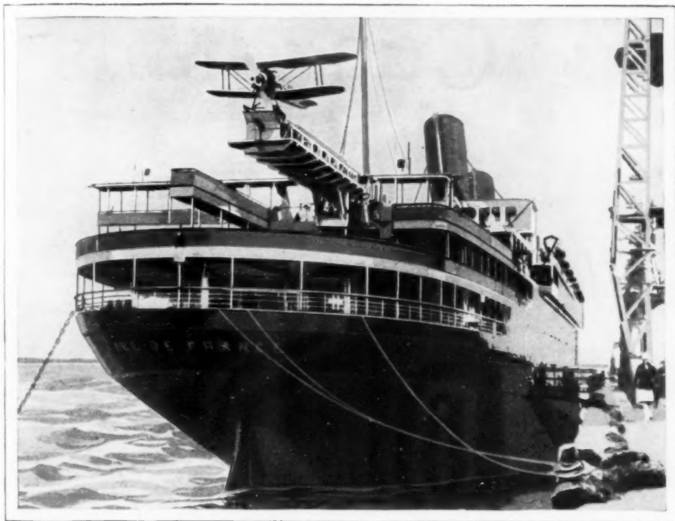
Catapult on Steamer "Ile de France" to Launch Planes; the Biplane Shown Here Was Superimposed on a Photograph of the Vessel
