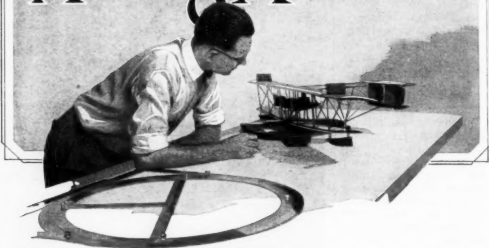
Examining a Model of One of the NC-Boats, the Navy's Flying Ship That First Crossed the Atlantic; Scale Models of Every Type of Airplane Are Built for Wind-Tunnel Tests
