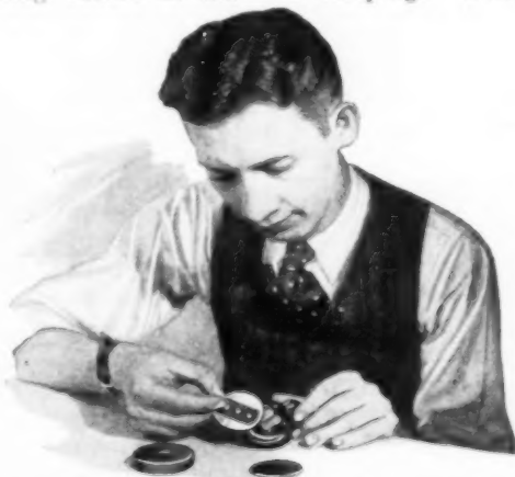
Phone Cap and Diaphragm Removed for Substituting Paper Disk and Razor Blade
