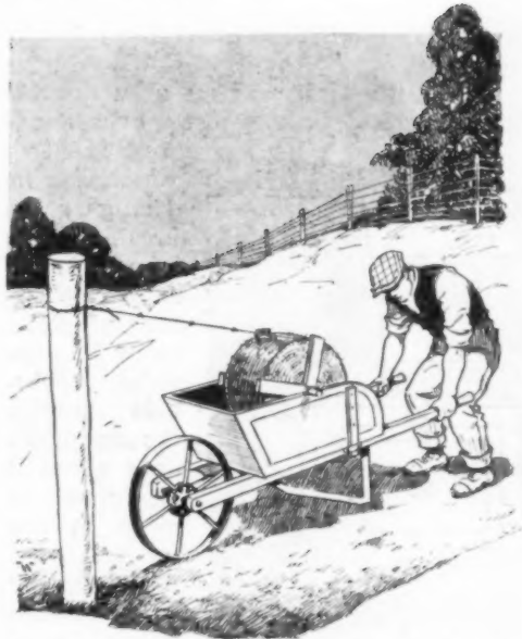
Barbed Wire Is Hard to Unroll Single-Handed but Easy with This Rig
