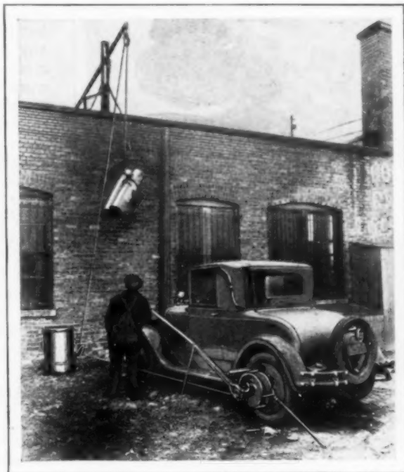
Auto Harnessed as a Hoist; Lowering of the Bucket without Reversal Is Done with the Lever Control
