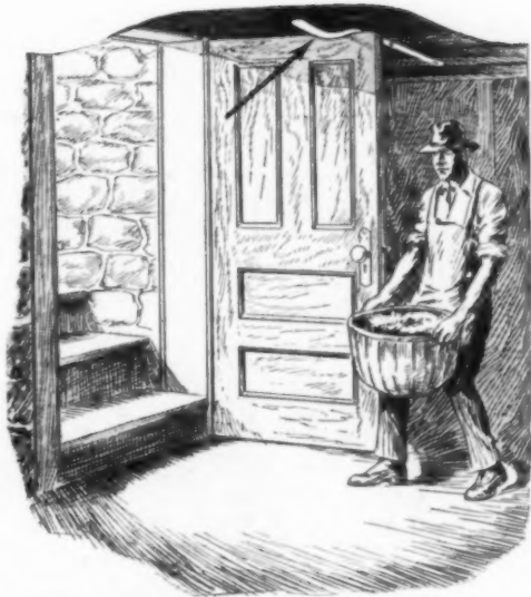
Spring-Metal Strip Nailed to Joists Holds Basement Door Open
