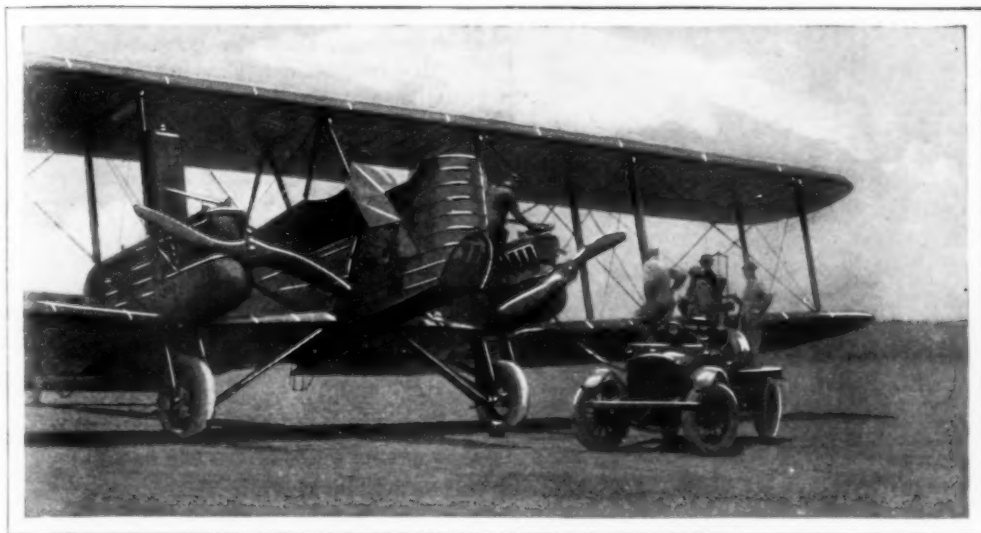
Filling the Gas and Oil Tanks of a Two-Engine Martin Bomber, One of the Biggest Planes the Cadets Learn to Fly; the Cockpit in the Nose Is the Forward Machine-Gun Nest
