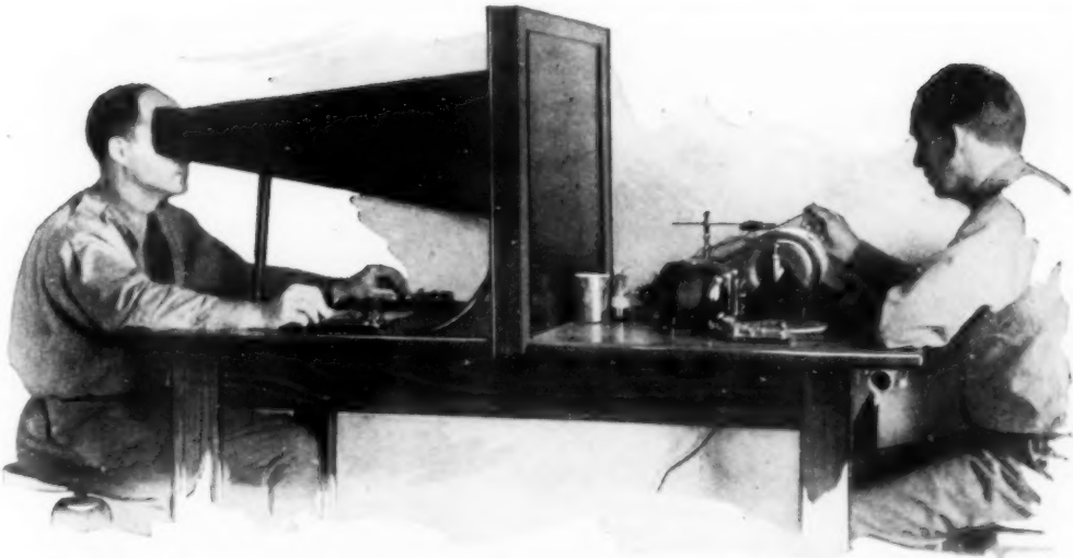
This Is the Reaction-Time Testing Machine, Which Measures the Interval It Takes the Hand to Respond to a Message Delivered through the Eye to the Cadet's Brain
