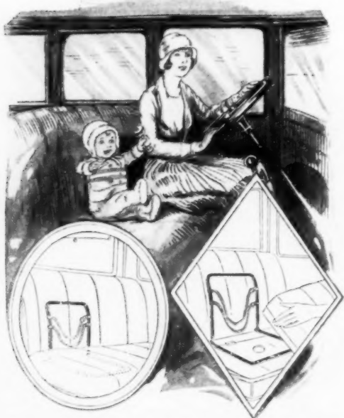
Seat in Place; How It Is Adjusted under Cushion, and in Use, with Straps about the Baby
