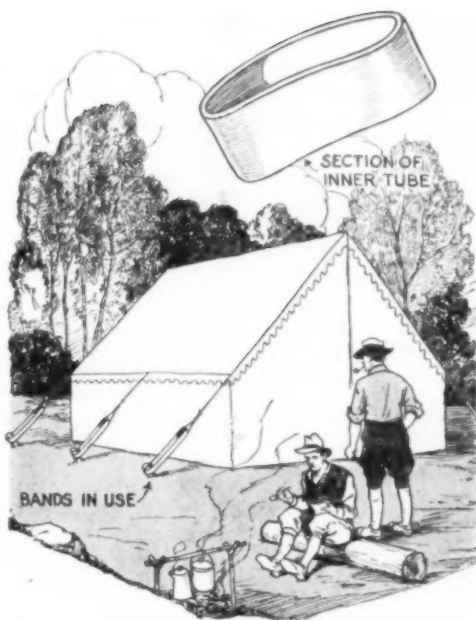
Elastic Stay Ropes for Tent Hold It Taut and Help Prevent Damage to Canvas
