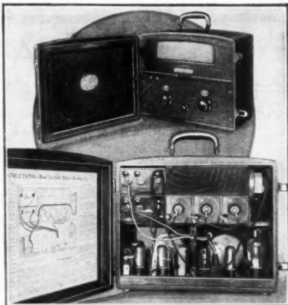
Front View Showing Portable Receiver Ready for Use; Below, Back Opened Showing Arrangement of Tubes and Batteries
