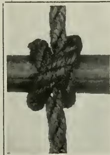
The Clove Hitch is a very safe knot, and may be handled very quickly
