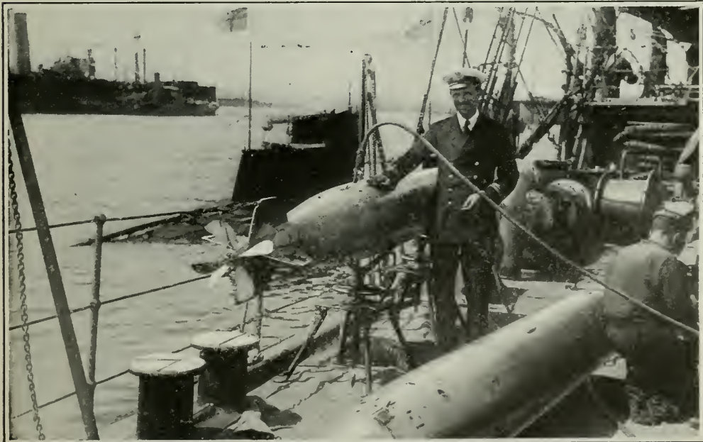
Torpedoes for the submarine in the background are being filled with compressed air at a pressure of one ton to the square inch. This compressed air runs the motor which sends the projectile at express speed, as well as the gyroscope spinning devices
