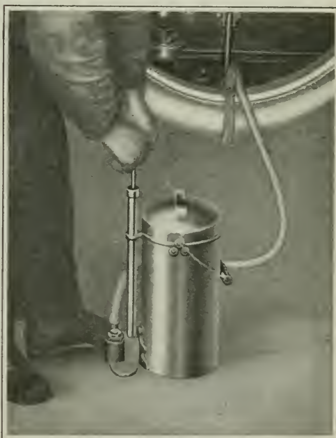
With one stroke a quarter-pound of grease is forced into the casing
