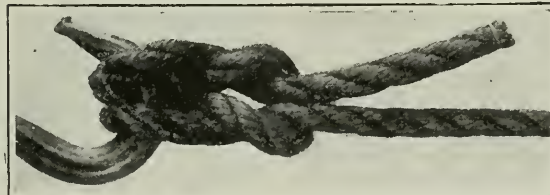
A "safety-first" tie, the Cat's Paw. This hitch will sustain heavy loads, and is most used for that reason
