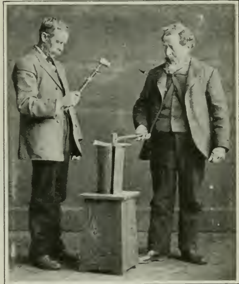
On the face of one hammer is a Maltese cross which is forced through the check when struck with the second hammer
