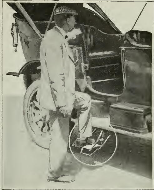
An automatic step lowered by pressure on a pedal. By its aid a small child may board the car with no great difficulty
