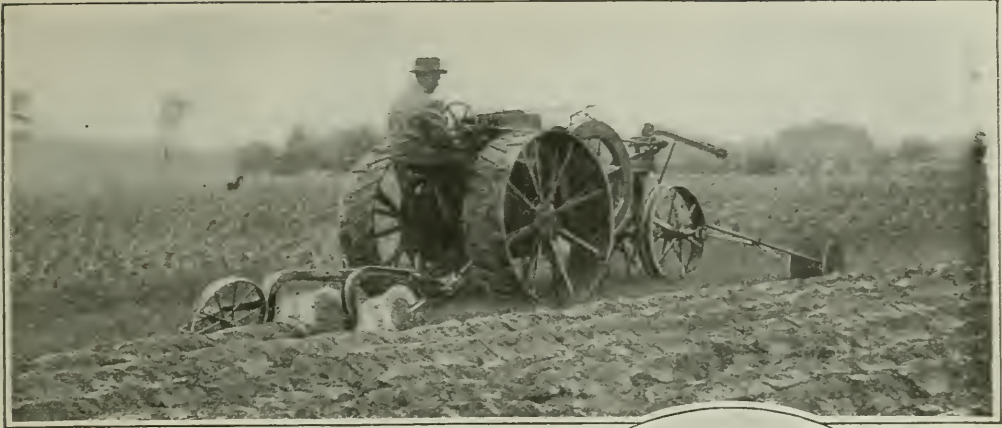
Above is an 8-16 horsepower tractor plowing sod. Note the self-steering attachment in front
