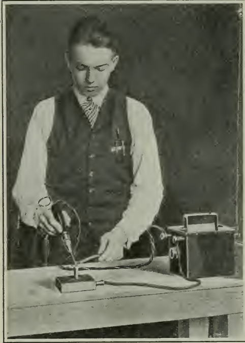
To obviate loss of heat by radiation, this soldering-iron has been invented. It heats the object to be soldered only at the point of direct contact
