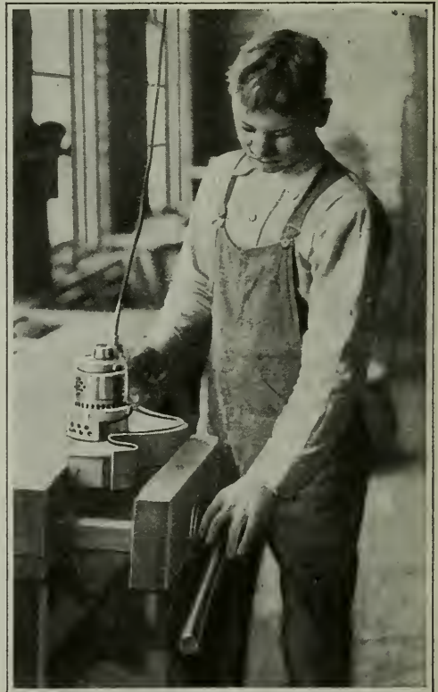
A boy can operate this electric planer (for it is nothing else). The concentrated power of electricity makes perfection easily attainable by the modern workman
