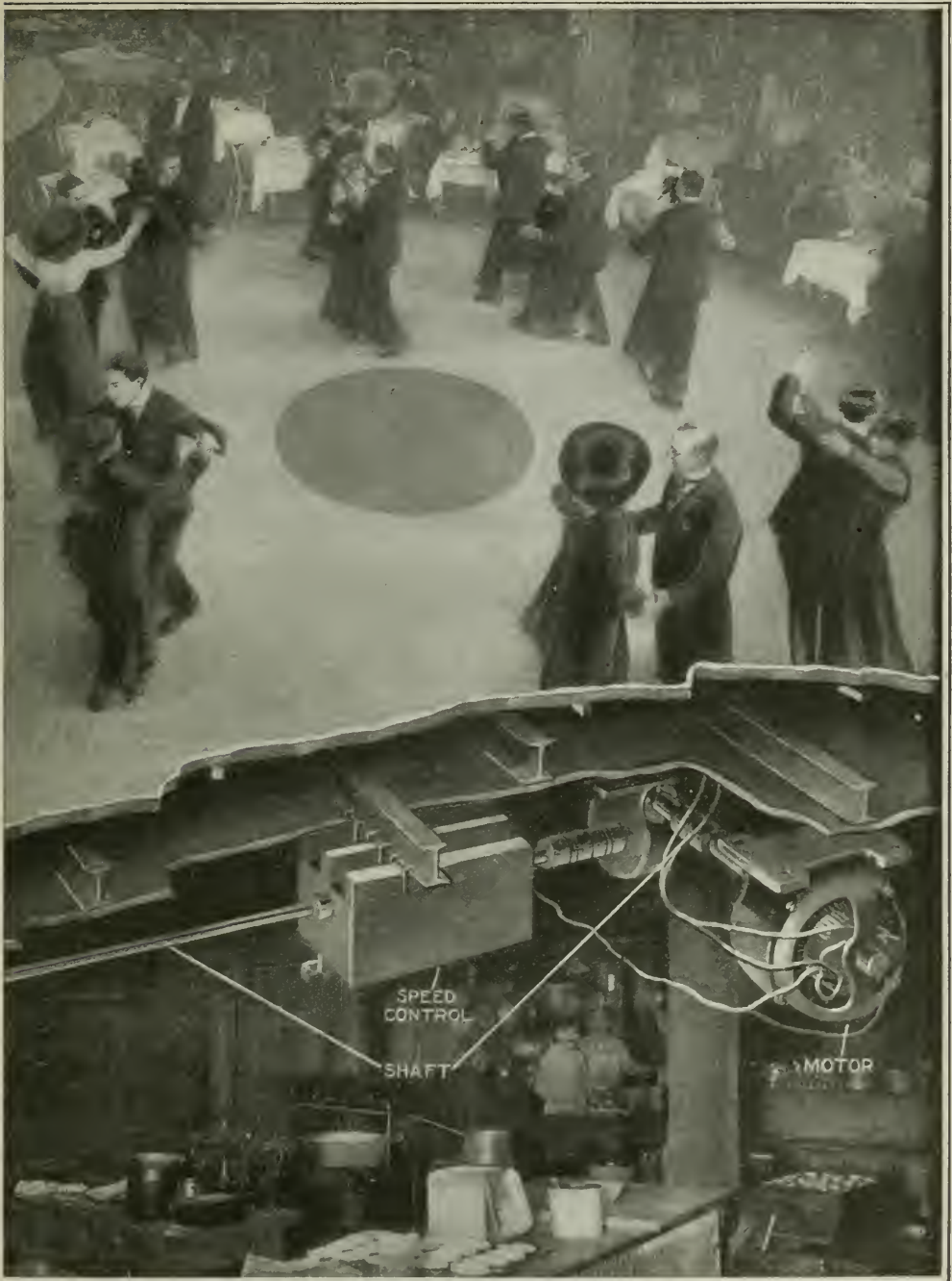
A New York restaurant is responsible for this newest development of the dancing craze. At first they tried to turn the floor at high speed, but this was found too fast for New Yorkers. Now the floor turns at a solemn but relentless rate. The whole floor, with as many as one hundred persons, is turned by a one-half horsepower motor, so well arranged is the mechanism
