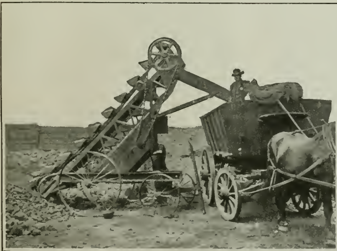
A loader which is built like a California gold-dredge and which can handle one cubic yard of crushed rock in a minute and a quarter
