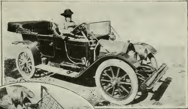
The "woman's fender" rolled up. In the oval, it is shown extended after the foot-brake has been depressed to meet an emergency; for the fender and brake are operated as a unit
