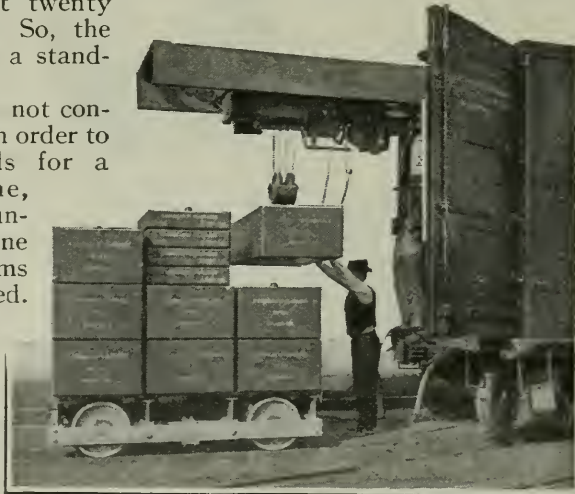
The test-car is used for detecting faulty railway scales
