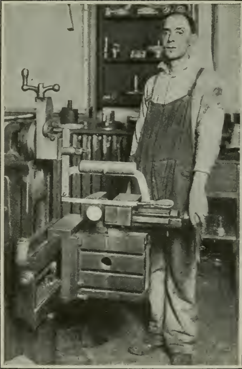
By means of this new attachment, a shaper is converted into a power hack-saw machine
