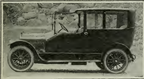
Handsome town landaulet. It can be opened rearward of the door with little overhang, as the roof over the window swings forward
