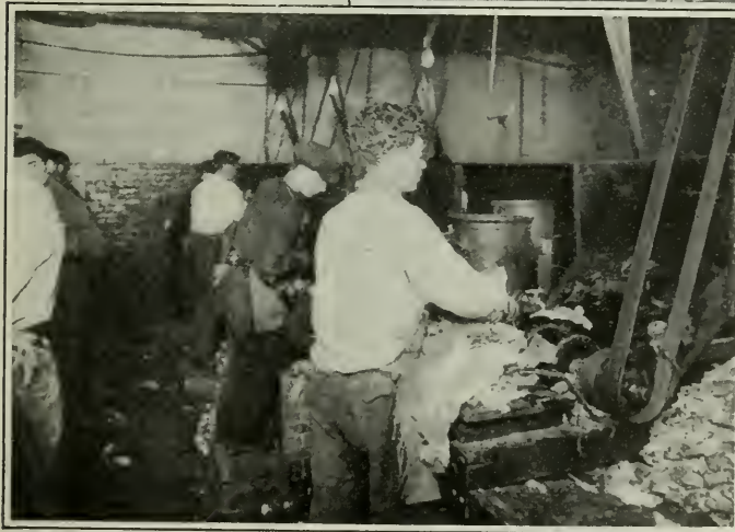
"Carroting," or scrubbing the rabbit pelts with nitrate of mercury solution. It is the use of this nitrate of mercury which constitutes the greatest hazard in the fur felt trade
