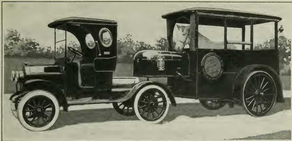
Every consideration is given to the injured horse in carrying him away to the hospital. This truck differs from the ordinary automobile ambulance in having a trailer
