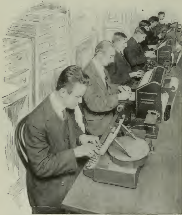
These eight operators work at one end of a single trunk line. Four are sending and four receiving, and they are kept busy every minute. The same number work on the other end of the wire, and it is possible to send more than six thousand messages over one wire in a single working day
