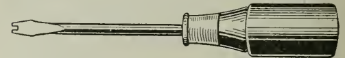
A notch in a screw driver gives a grip on wires to be twisted around binding posts or sockets
