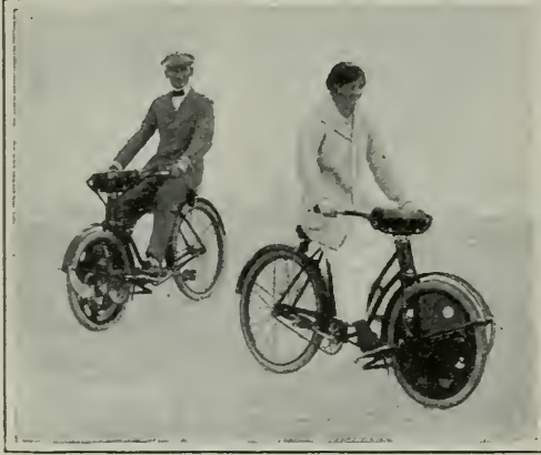
This front-wheel drive motor-cycle will run one hundred miles on one gallon of gasoline
