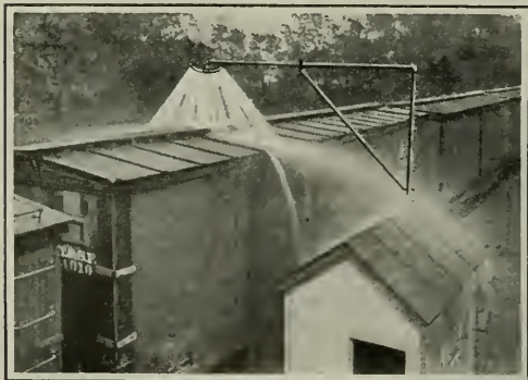
This railroad does not wait for a damage suit to learn whether or not a car roof leaks
