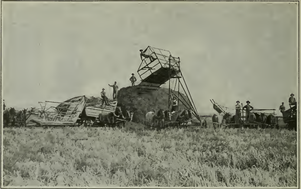
A rope drawn by horses lifts the load to the desired height. Then a clutch is released, the platform tilts, and the straw slides off
