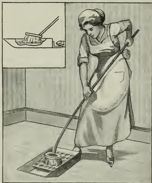
Dust from the mop falls through the sieve and is caught in the dustpan
