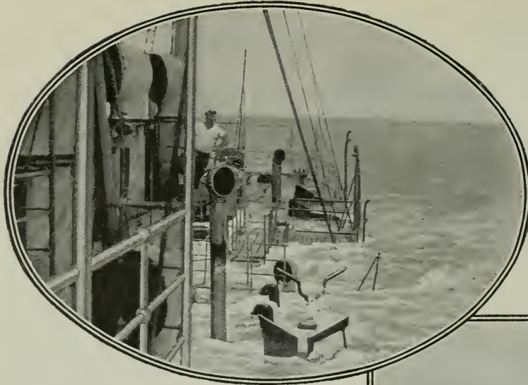
The ship had been sunk on a bar in the open roadstead, so that the upper works were awash. The surging of the rollers and the undertow made it difficult for the divers to work or to move about
