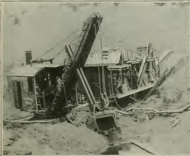
The dredge gulps from six to twelve hundred cubic yards of gold-laden dirt every day
