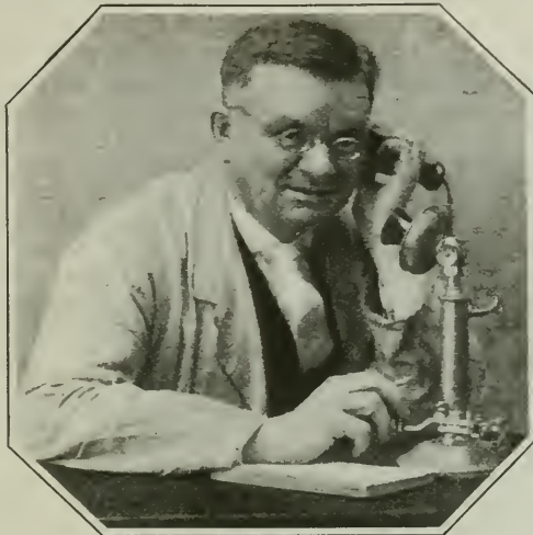
A telegraph-key attached to a telephone, which places the whole vast telephone system of the country at the disposal of the telegrapher
