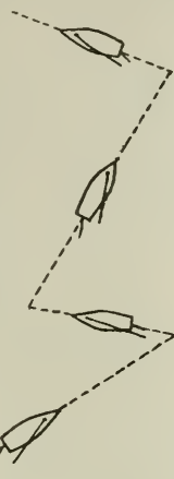
If the wind is not "dead ahead" the "tacking" must be irregular
