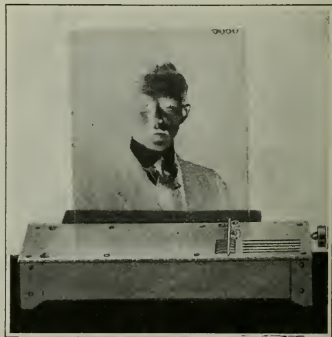
Transparent numerals on a small opaque area or opaque numerals can be transferred to each negative
