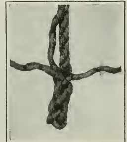
The second operation in preventing the dead end of a rope from ravelling
