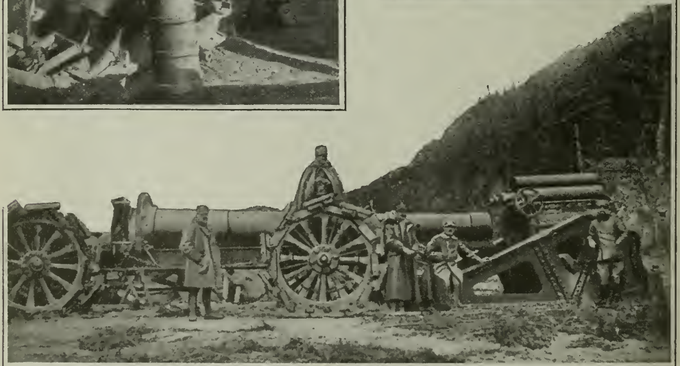
The Italian engineers have proved themselves among the best in the world. Time and again the Austrians have been surprised by having shells dropped upon them, apparently from the skies. The Italians had dragged huge guns up precipitous mountain slopes and were safely installed out of the enemy's range on plateaus, from which shells were fired over mountains. Here we see a 305-millimeter gun (12-inch) being assembled on a mountainside
