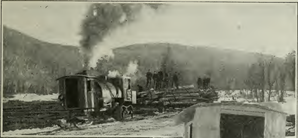
A steam tractor helps reduce logging costs in the Maine forests. Caterpillar wheels support the tractor on the snow
