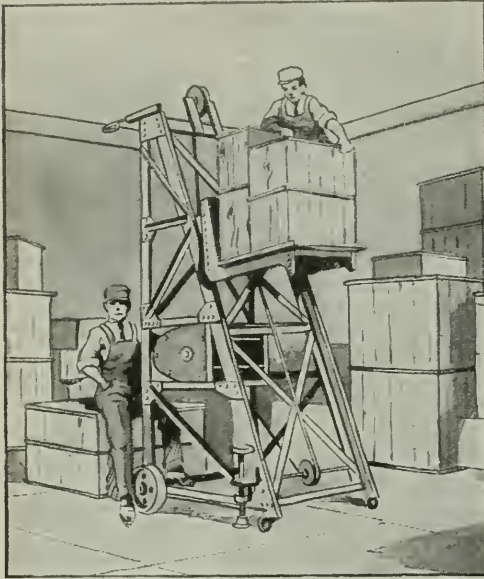
Boxes and bales for storage are easily handled by two men with this simple movable elevator
