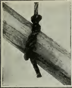
The Timber Hitch, a safe and simple knot usually employed in holding poles and booms. The turns in the loose end must be carefully made
