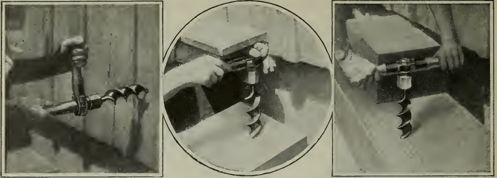
A new auger which will work in any position and around almost any obstruction. It can be used in a corner, under a shelf, or even inside a box with equal facility
