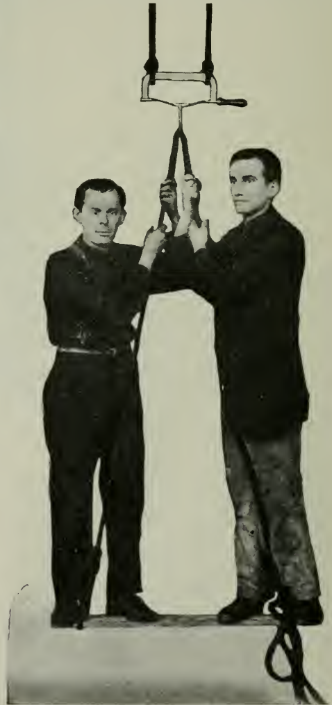
The thin hack-saw, although bending badly, is supporting two hundred and eighty-two pounds without damage to itself
