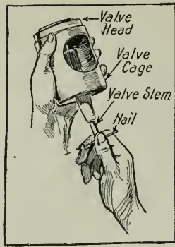
Fig. 12. A nail or piece of wire will grind Buick valves
