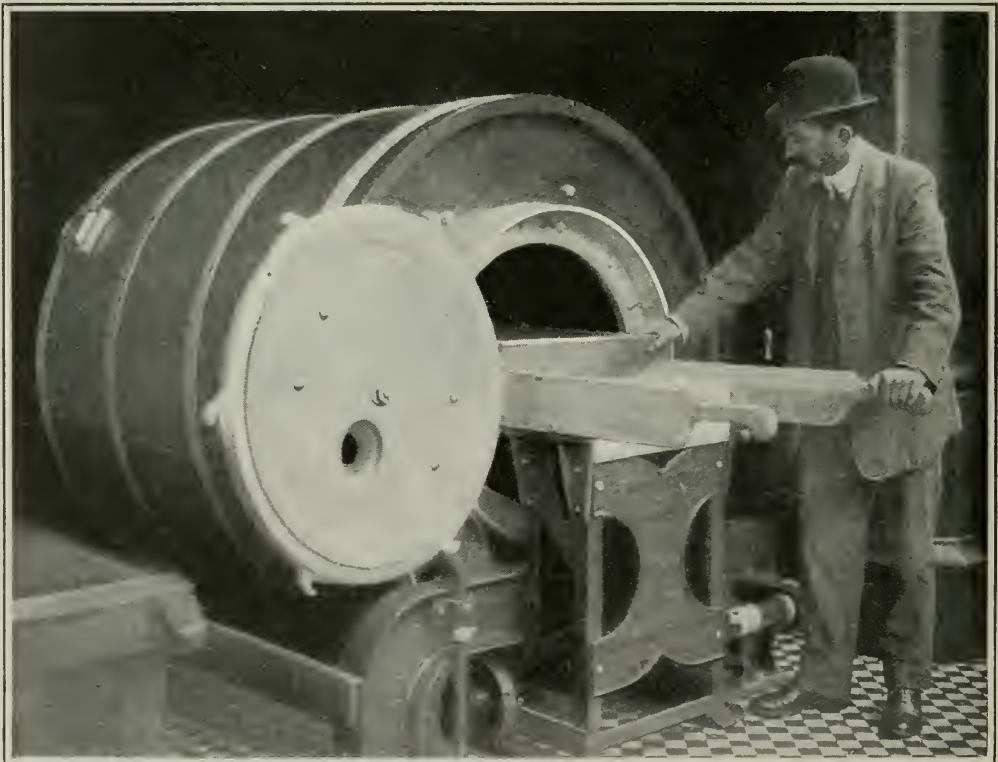
This monster churn makes and washes six hundred pounds of butter at a single operation, and is exceeding valuable at this time in English hospitals, where wounded soldiers consume large quantities of dairy products by the orders of their doctors
