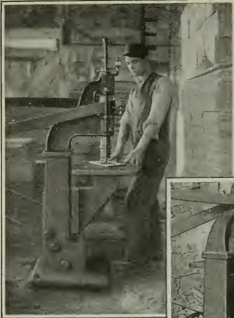
A machine which cleans out knot-holes and then plugs them with a solid piece of wood
