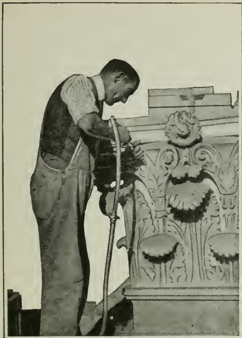
This pneumatic chisel is installed in the sculptor's studio, and greatly simplifies his work
