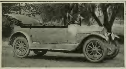
Open position of above body. The enormous mass of the top when folded down is unfortunate. Otherwise a most successful design
