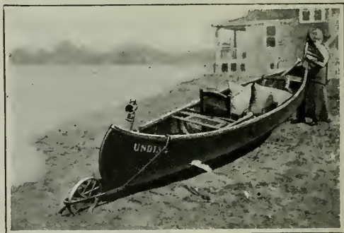
With a wheel on the front, a canoe can be handled easily by a woman or child
