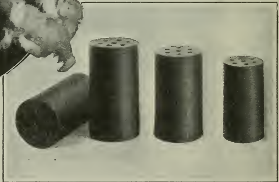
Cotton nitrated and ready to be transformed into smokeless powder (nitrocellulose). Grains of smokeless powder (nitrocellulose) are perforated so that they can burn inside as well as outside, thus controlling the rate of gas production
