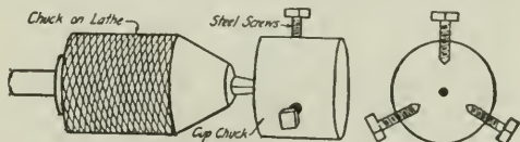
A good substitute for a scroll chuck
