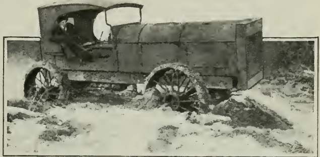
This four-cylinder tractor develops sixty horsepower, which is divided between front and rear axles, affording great tractive ability
