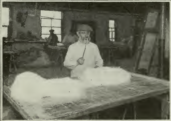
A fur worker beating fur by hand. The workman is not protected from the particles of fur and dust which are raised by his beating
