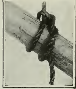
The Timber and Half Hitch. Much the same as the Timber Hitch with the addition of a half hitch to avoid any danger of the rope's rolling
