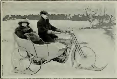
A motorcycle on runners is a novelty, but its practicability has been proven
