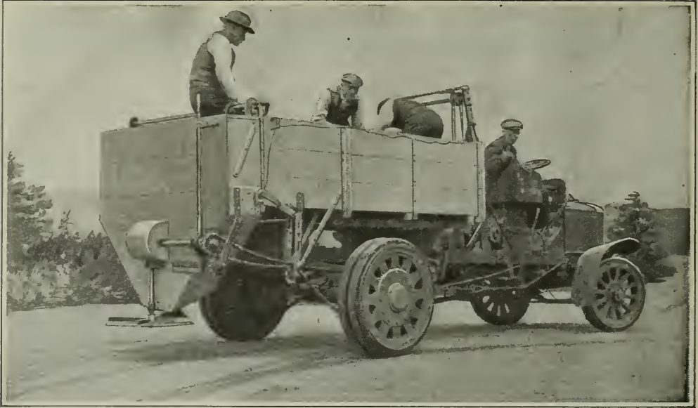
Revolving fan blades beneath the hopper of this sand truck throw the sand over many feet of street surface which has been freshly oiled
