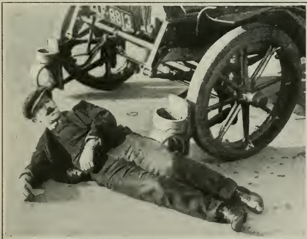
The rubber guards strike the body and gently tosses it to one side away from the heavy wheels
