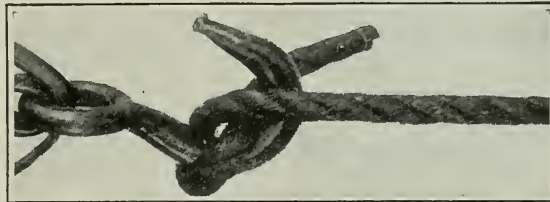
The Blackwell Hitch, while safe for light loads, is likely to part under heavy strains
