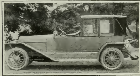
Closed position of French double phaeton landaulet. An extension top (not shown) covers the driver. Taper of hood changed from stock model (above)
