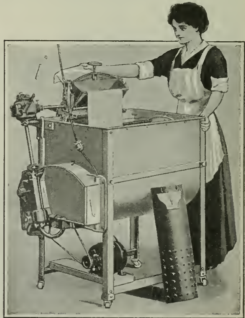
The need of a guard to prevent injury to the fingers in an electric wringer has been met by this device
