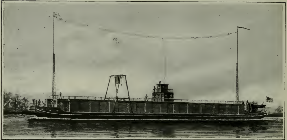
Motor-barges equipped with traveling-cranes, wireless apparatus and other modern apparatus, are to supplant the romantic Mississippi stern-wheeler
