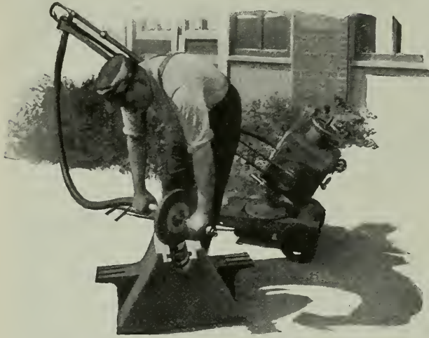
The newest thing in portable tools is a grinder which goes to the blade to be sharpened
