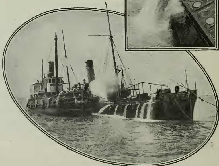
When the "Progreso" was pumped dry, she was able to steam to Vera Cruz, where she was dry-docked and thoroughly examined
