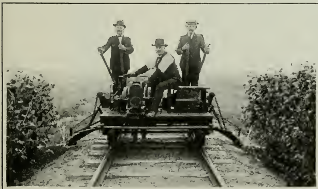
Three men on this motor hand-car can mow as many weeds in a day as a hundred men working in the old way
