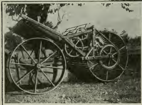
The newest fruit picker is a roller which lifts the fruit up from the ground after it has fallen from the tree
