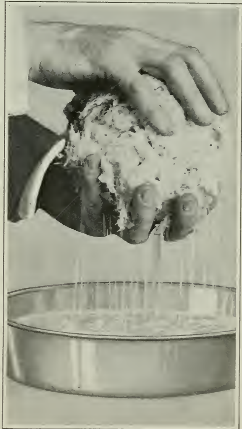
A handful of "Sauerkraut," not the real thing, but the kind used for fuel. It is really wood pulp, the rejected portion of a paper mill's product
