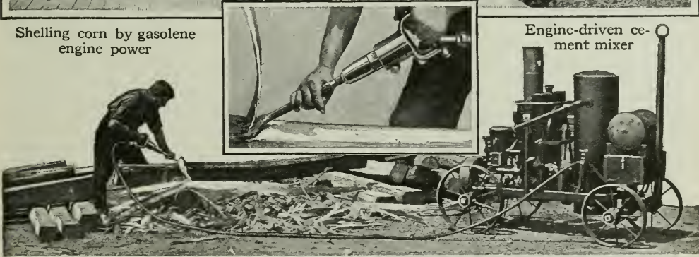
A portable engine driving an air compressor operating a pneumatic timber stripper
