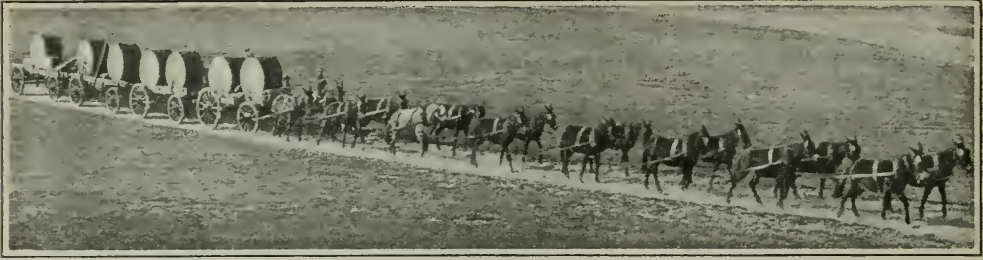
Four four-mule teams are more efficient when pulling together than when separate where extensive transportation is necessary. The maximum traction effort required is less than four times the maximum for a single team
