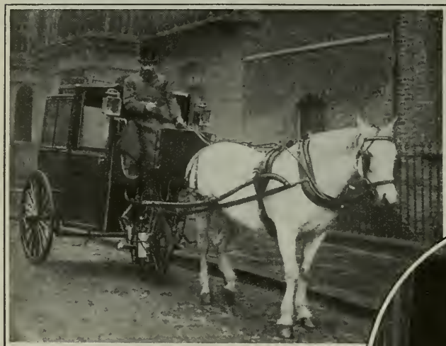
A London cabby designed this three-wheeled cab. The third wheel prevents the cab from tipping over, even when making the shortest and quickest of turns
