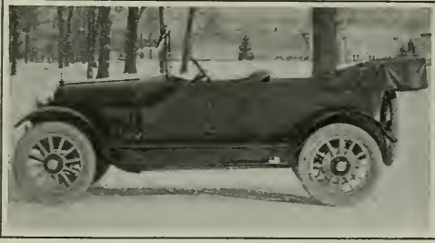
Wheelbase is too short. Front seat with its imitation of a double cowl cuts down effective opening of rear door. Back mudguards poorly designed
