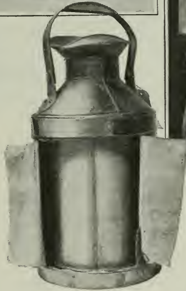
The purchaser of gasoline sees only the five-gallon measure, but the three-gallon measure inside is the one really filled
