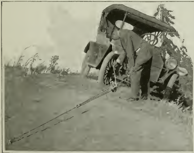
Turning the crank exerts seventy times as much power as the force applied, so that the car is easily dragged out of the ditch or up an embankment
