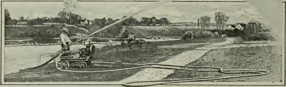
The portable gasoline engine makes possible the watering of lawns and parks where the source of water supply is a nearby lake or stream
