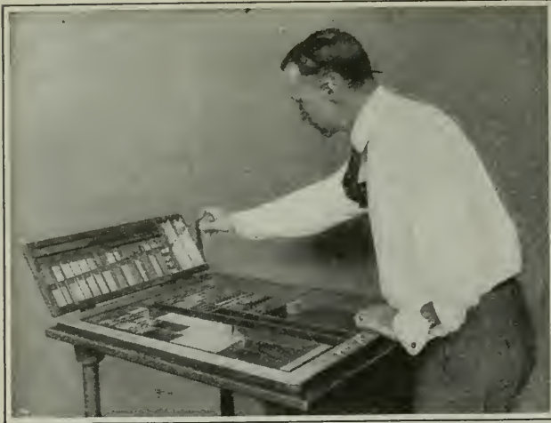
The type furniture awaits the make-up man in a rack attached to the "turtle" table
