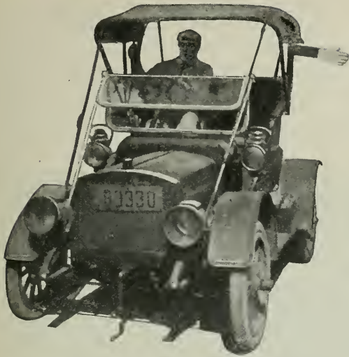
This driver need not lean out to signal an off-side turn. The artificial hand saves him that trouble
