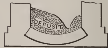
FIG. 8. OLD LONDON "SEWER OF DEPOSIT."
